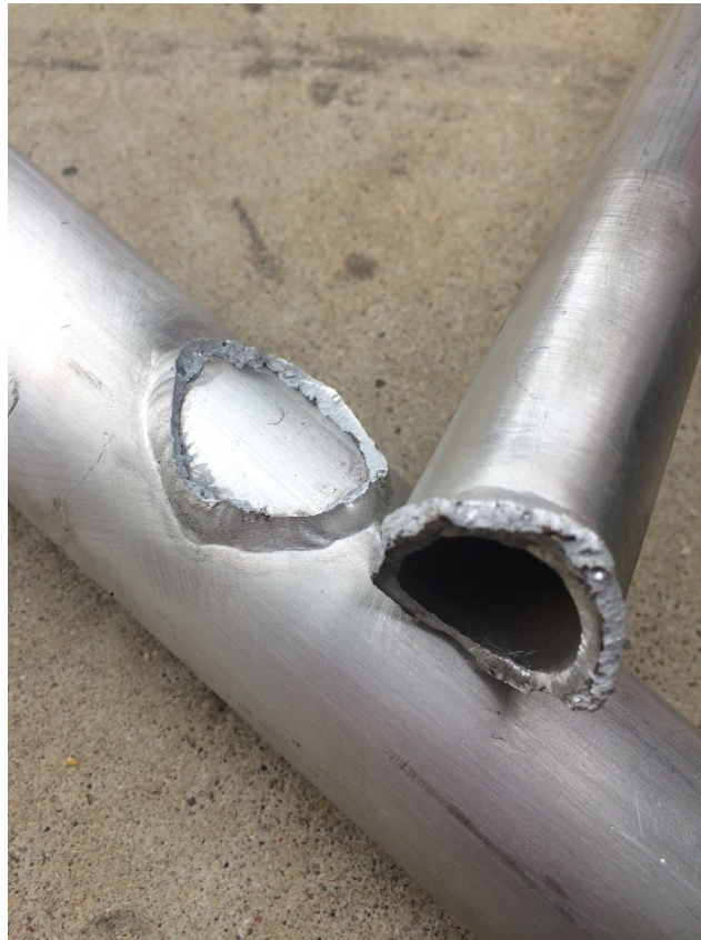
Figure 4.1.1: Demonstration on how the strength of an aluminum weld is governed by the filler material.
