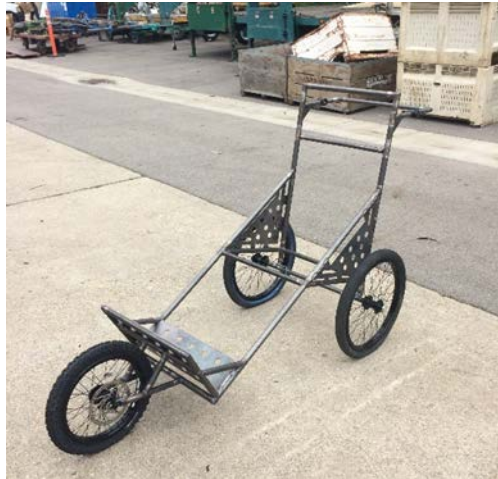
Figure 5.1.6: The finished frame before paint
