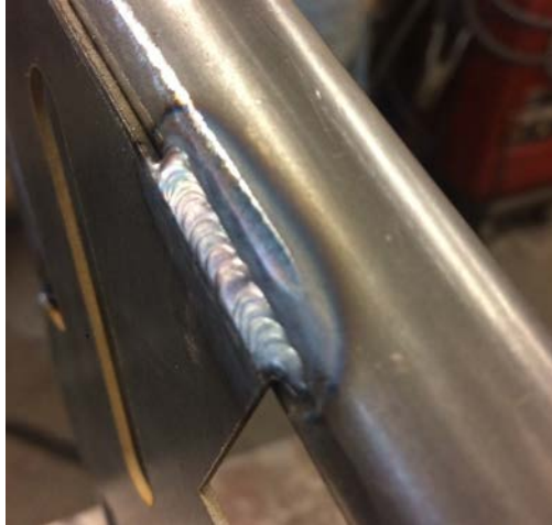
Figure 5.1.5: An example of the Tig weld quality on the frame
