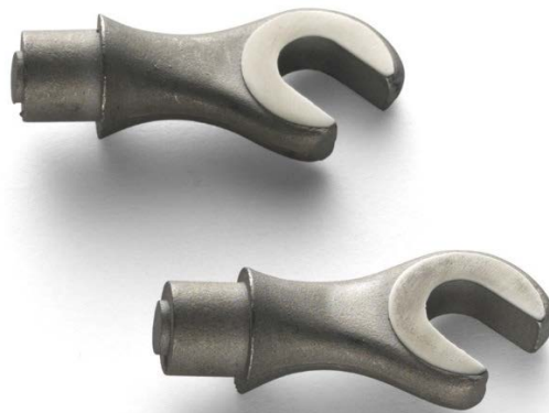
Figure 4.5.4: Standard Bicycle QR accepting front dropouts. Made out of steel that can be easily welded to bond with 4130 chromoly tubing.
