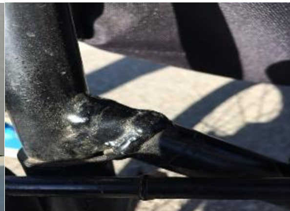
Figure 2.1.3: Repair Weld on Joseph's jogger
