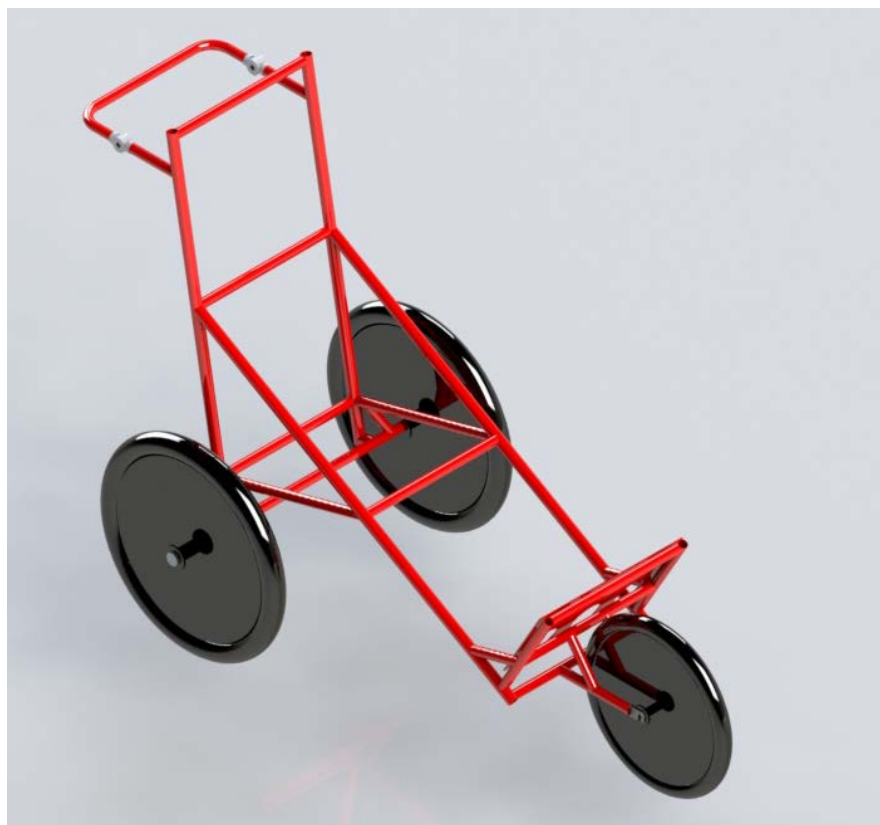
Figure 4.1.2: Final frame design made with high strength 4130 Chromoly steel tubing.
