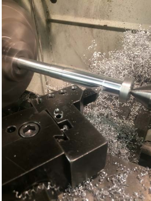
Figure 5.4.1: Machining of one rear axle shaft on a manual lathe in the hanger.
