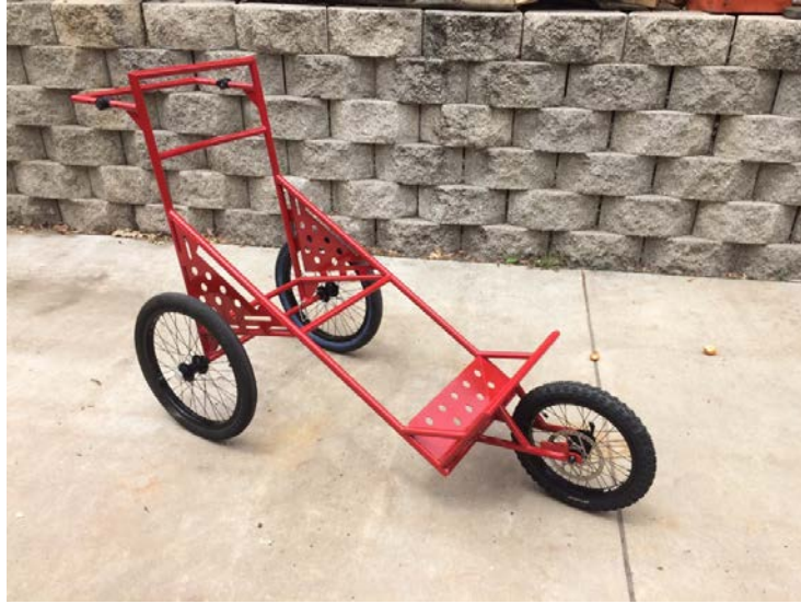
Figure 5.1.7: The completed frame fresh out of powder coating.
