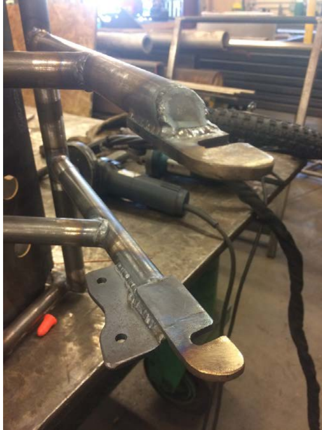
Figure 5.4.2: Finished drop outs welded to the frame. In order to ensure correct spacing between them when welded, a 100mm spacer was put in-between when they were tacked on. The disc brake mount is shown on the lower fork leg.
