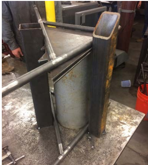
Figure 5.1.3: Makeshift Fixture used to align both sides of jogger frame.
