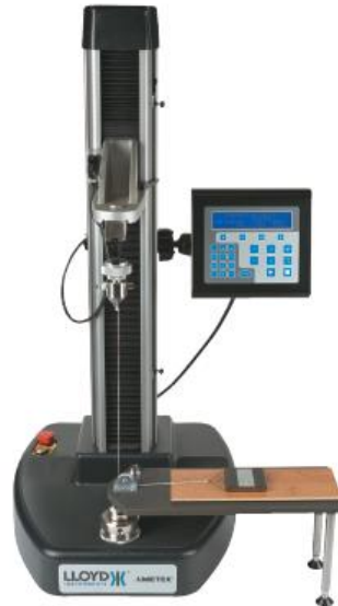
Figure 1. Lloyd Materials Testing FT1 Friction Test Machine [1]
