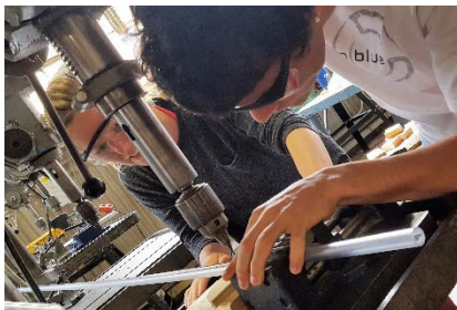
Figure 29: Donovan and Dakota drilling holes in a clear PVC pipe
