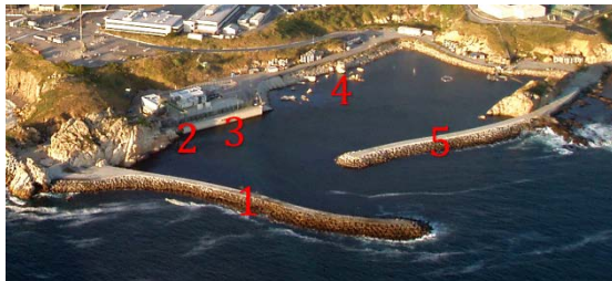
Figure 3: Visual of intake bay. 1 notes west breakwater, 2 notes Unit 1 intake, 3 notes Unit 2 intake, 4 notes rock with permanent chain, and 5 notes east breakwater.
