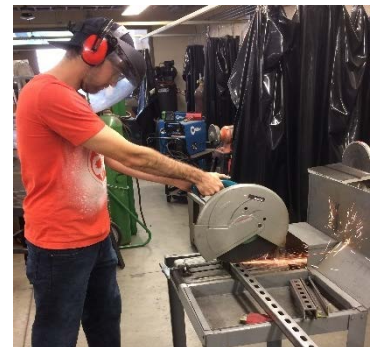
Figure 28: Christian using a Miter saw to cut the Unistrut beams
