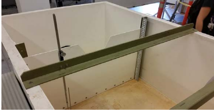
Figure 24: The weir box in the 192-102 fluids lab. This picture is before alterations were made; the weir plate no longer exists and tank can be filled to full height.
