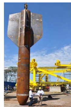
Figure 14: A large torpedo anchor, used mainly to anchor oil rigs.
