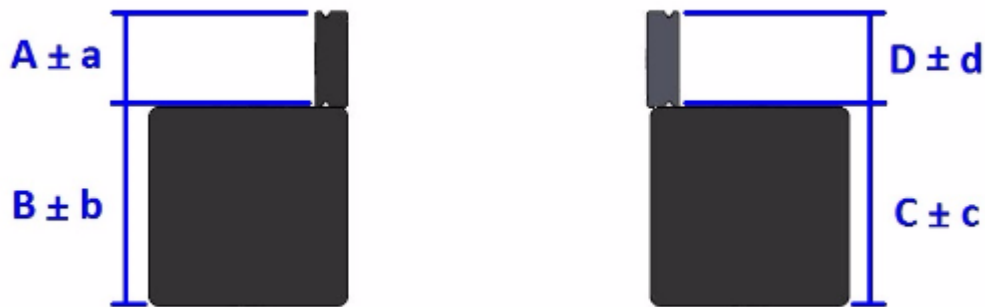
Figure D4.2. Schematic of tolerance stack up for beam to rail analysis showing rail ( A \pm a ), granite parallel ( B \pm b ), granite parallel ( C \pm c ), and rail ( D \pm d ).
