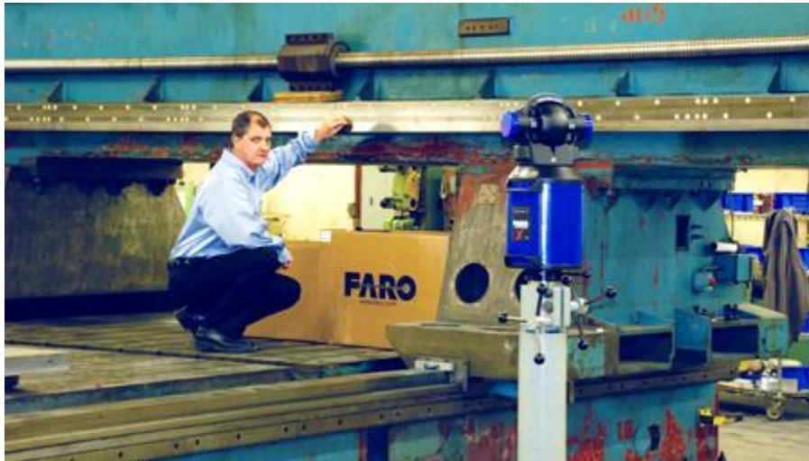
Figure 4: FARO Laser Tracker for linear rail alignment. The blue cylinder is the actual laser system while the device the subject in the photo is holding is the other part of the system for measurement. This image is courtesy of FARO.
