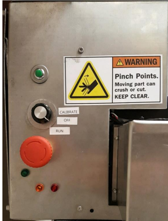
Figure 1. User Interface Panel Buttons from which the user will control the operations of the XBAS. The XBAS should be positioned so that the user can easily access these buttons.
