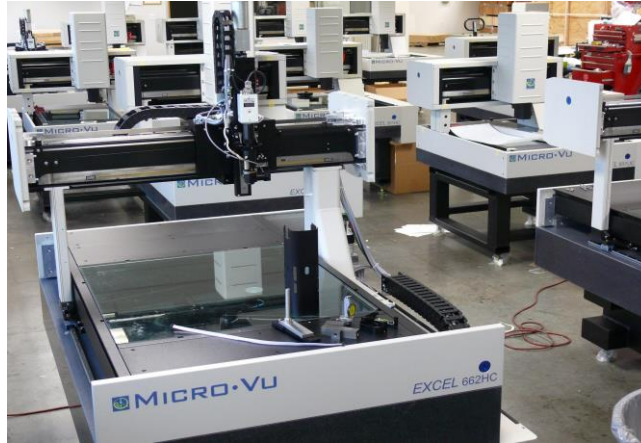
Figure 2: Micro-Vu Excel Machine. The Micro-Vu Excel is one of their best-selling precision measurement machines. It performs precise and accurate measurements using a camera and light system.
