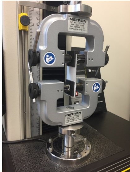
Figure 26. Test sample of TPU used in Instron pneumatic side action grips.
