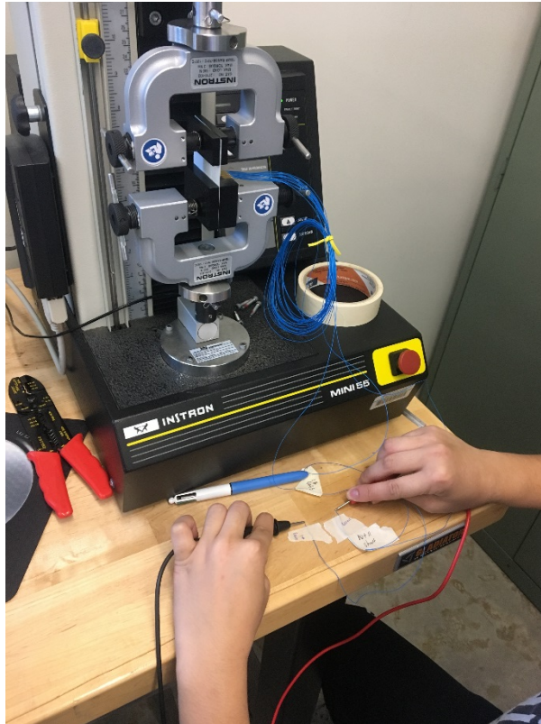
Figure 44. Test set up for verification testing when resistance monitoring was required. In this picture, the wires were being held manually to the multimeter. In later tests, the wires were attached to the multimeter probes with electric tape to ensure a more reliable connection.
