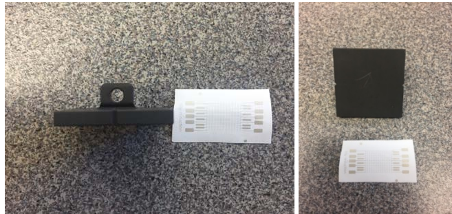
Figure 19. Photos of sample and flat Instron clamp for scale. Examples of stock Instron steel plate clamps that could be used with an external monitoring system.
