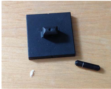
Figure N12. Instron flat face clamp and 1/8" Instron locking pin.
