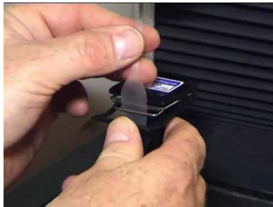
Figure 5. Instron thin film grips for 25mm specimen width (catalog no. 2713-006) [3].
