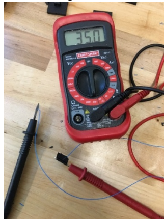
Figure N21. Example of terminal wires of interest attached to multimeter.
