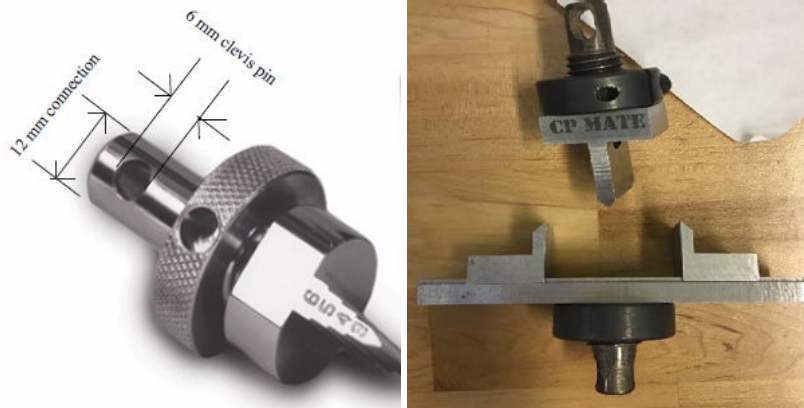
Figure 4. Left: Examples of Instron connection and clevis pin dimensions [3]. Right: Accessory used by the Cal Poly's MATE Department to perform 3-point bending tests. Fixtures such as this will be made in order to perform a variety of tests on FHEs. Personal photograph by author.
