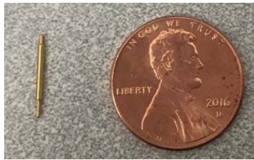
Figure 27. Sample of Emulation Technology Inc. Ultra-Mini Pogo Pin with recommended installation pitch of 1.0mm.
