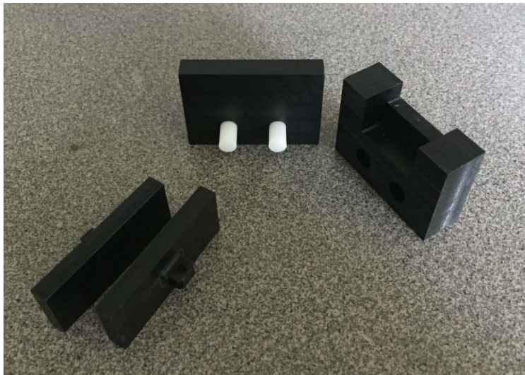
Figure 38. CNC-milled top blocks, alignment block, and U-block. Note that the dowel pins have been press fit into the alignment block after machining.
