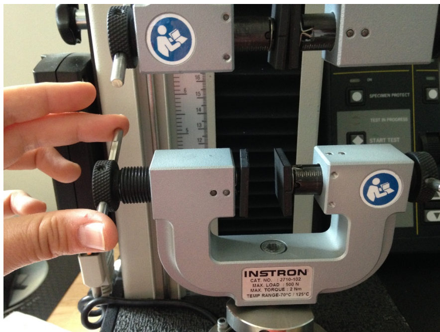
Figure N10. Twist side action jaws until flat clamps fall out.
