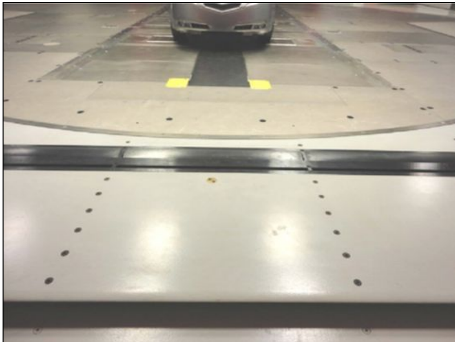
Figure 5. Honda Scale Model Wind Tunnel two-stage boundary layer removal system
