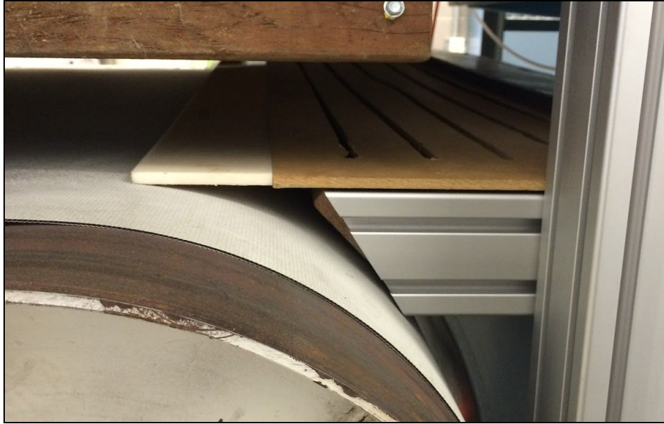
Figure 25. Fully assembled device flush against rolling road. Note that the rolling road is not raised to the height of the tunnel floor
