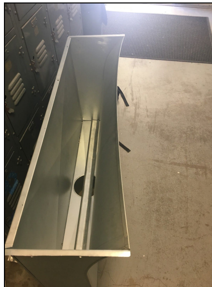
Figure 20. Plenum warping without addition of structural brace
