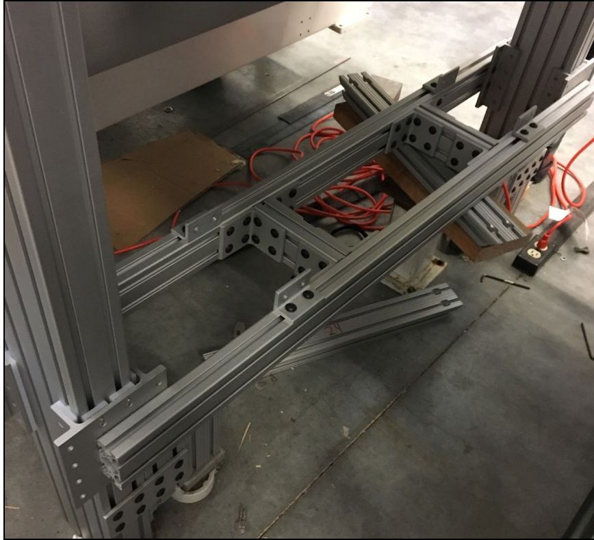
Figure 24. Fully-assembled framing subsystem
