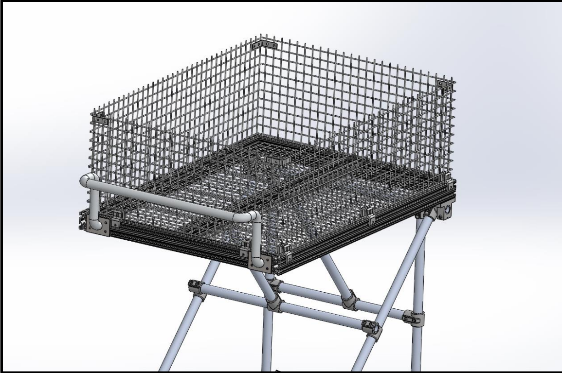
Figure 39: The basket & handlebar subsystem for the 80-20 T-Slot frame
