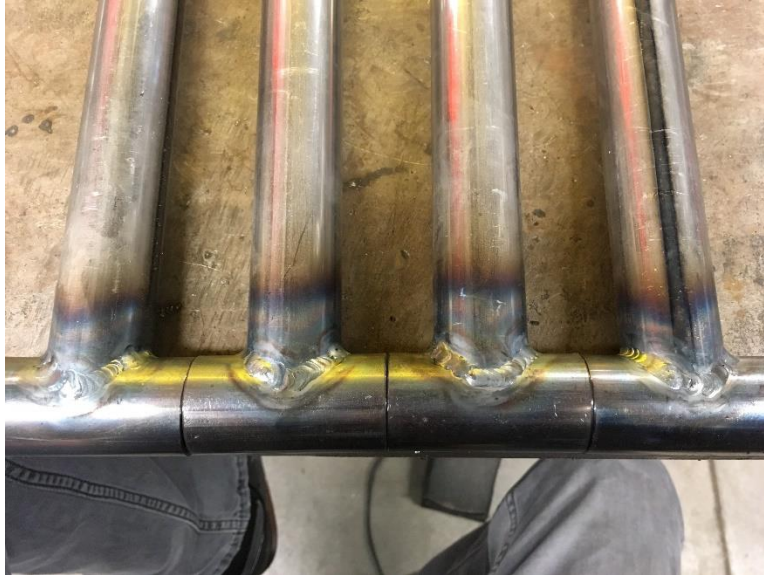
Figure 53. 90-degree tubing welded into place for leg hinges
