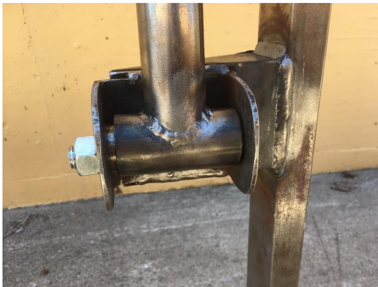
Figure 54. Assembled hinges with all components in place
