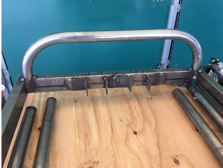
Figure 52. Handle bar bent, cut, welded into place
