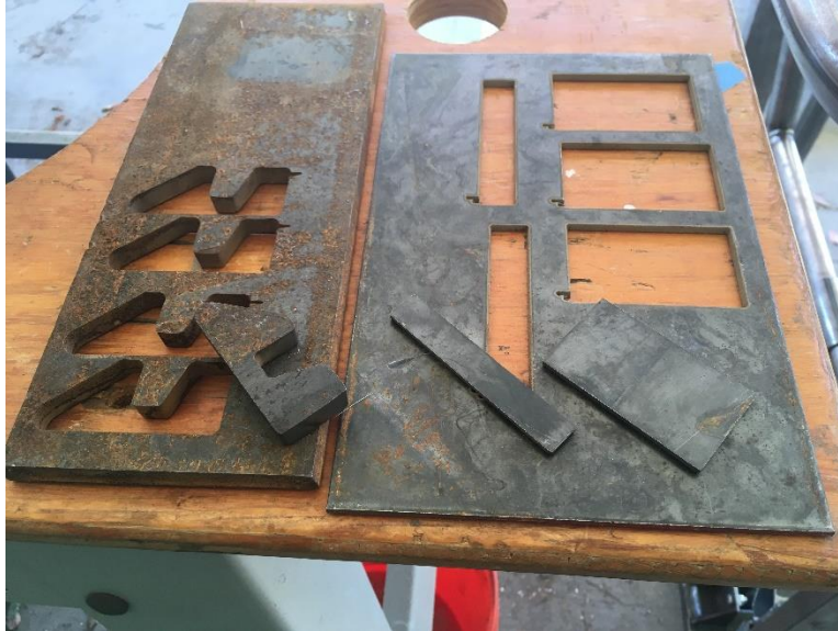
Figure 60. Locking mechanism pieces cut using the water jet
