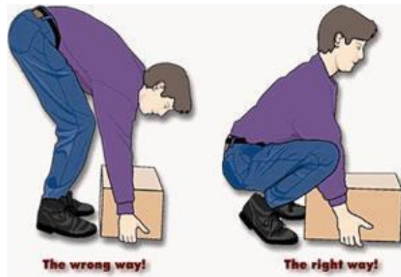
Figure 21: Improper Lifting Technique [21]
