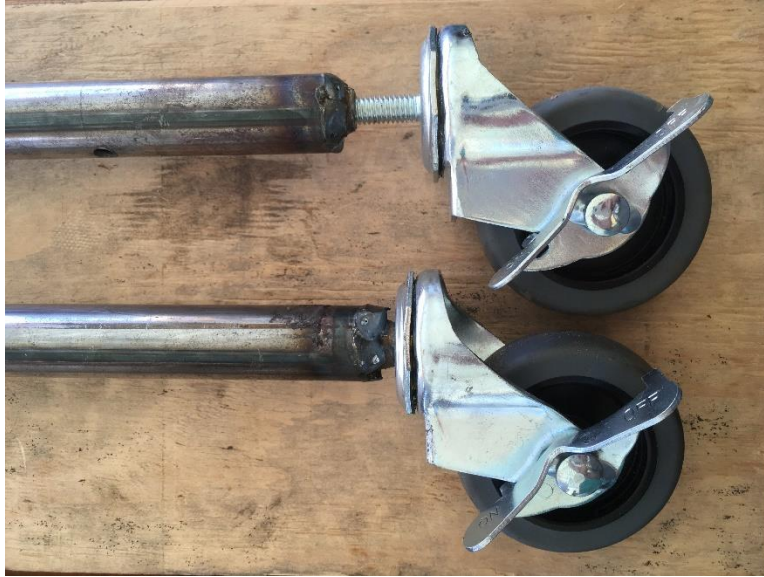
Figure 56. Lower legs welded with nut insert and threaded rod casters attached
