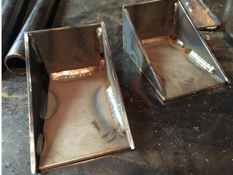
Figure 50. Supporting brackets to mount hinge brackets to frame
