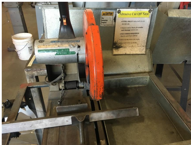
Figure 47. Chop saw cutting stock length material
