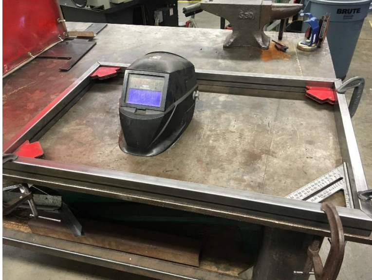
Figure 48. Clamping and fixturing in preparation for frame welding
