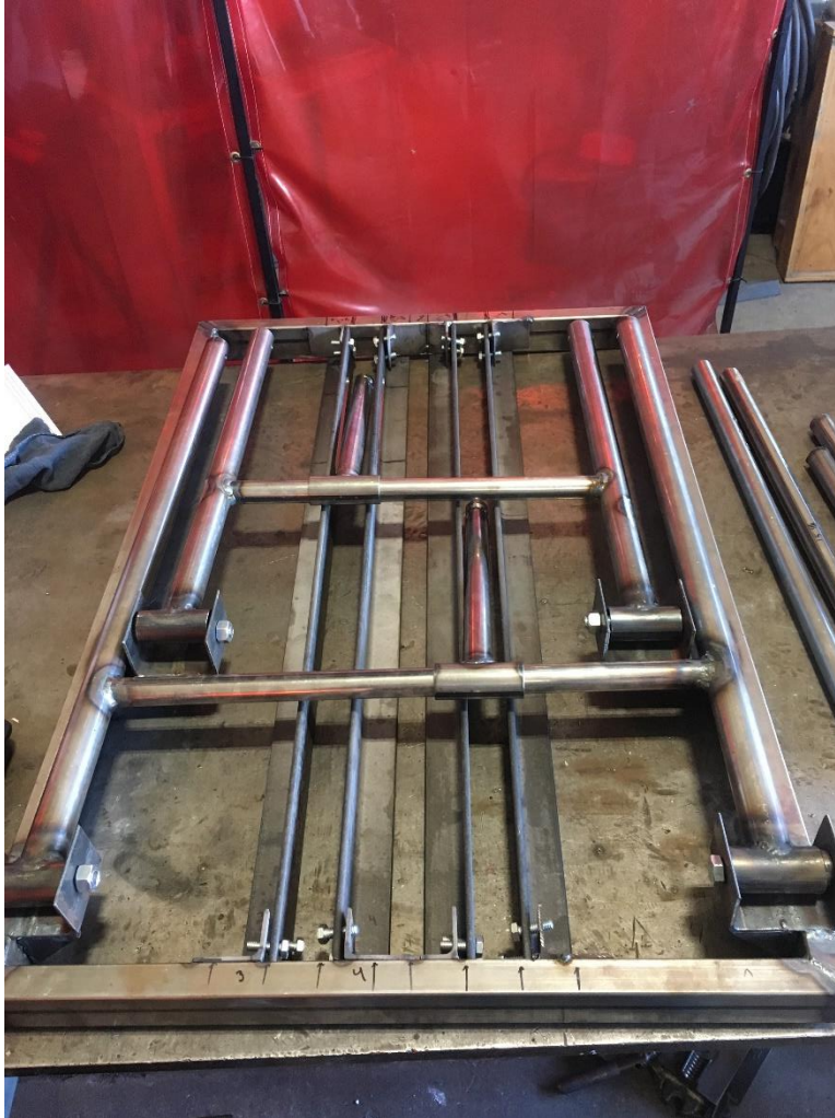
Figure 59. Sliders and leg assemblies test fit on frame
