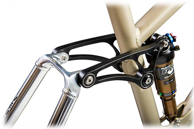
Figure 4. CNC machined aluminum rocker arms on a Ventana USA bicycle [7]
