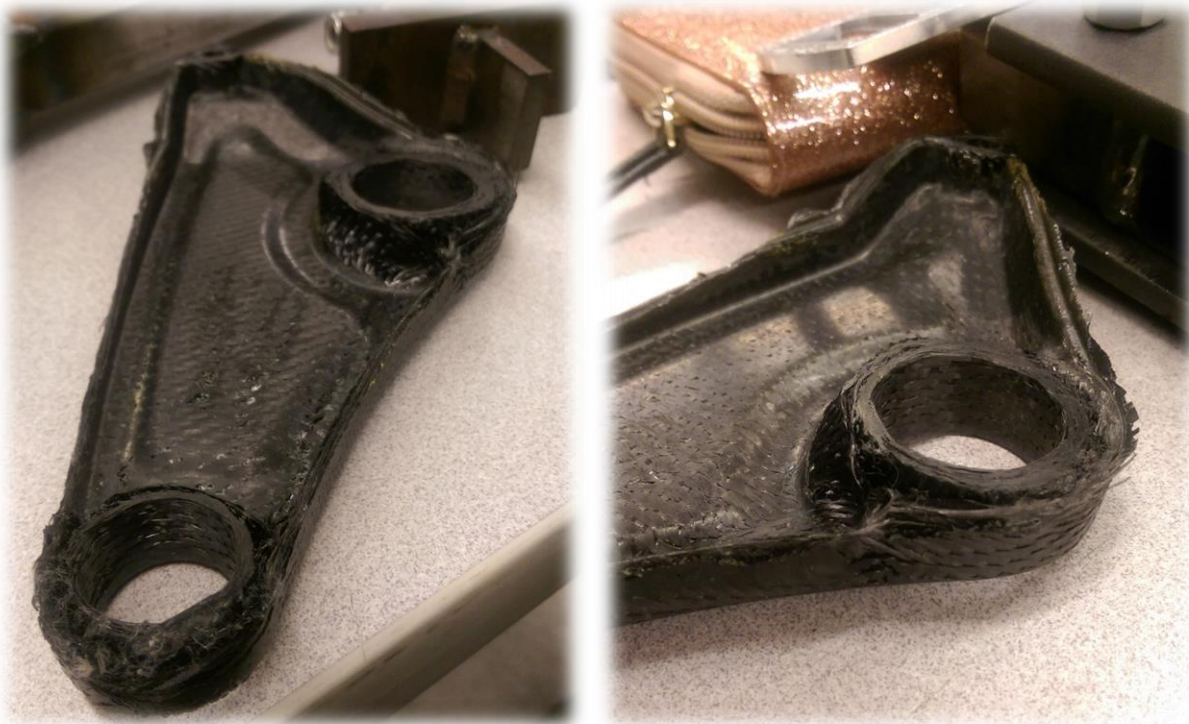
Figure 39. First rocker produced, showing signs of low compression, not enough fiber, and low resin content.
