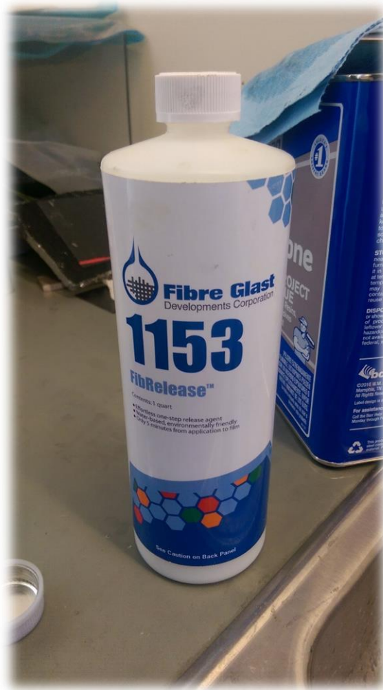
Figure 37 FibRelease used as the release agent for the mold
