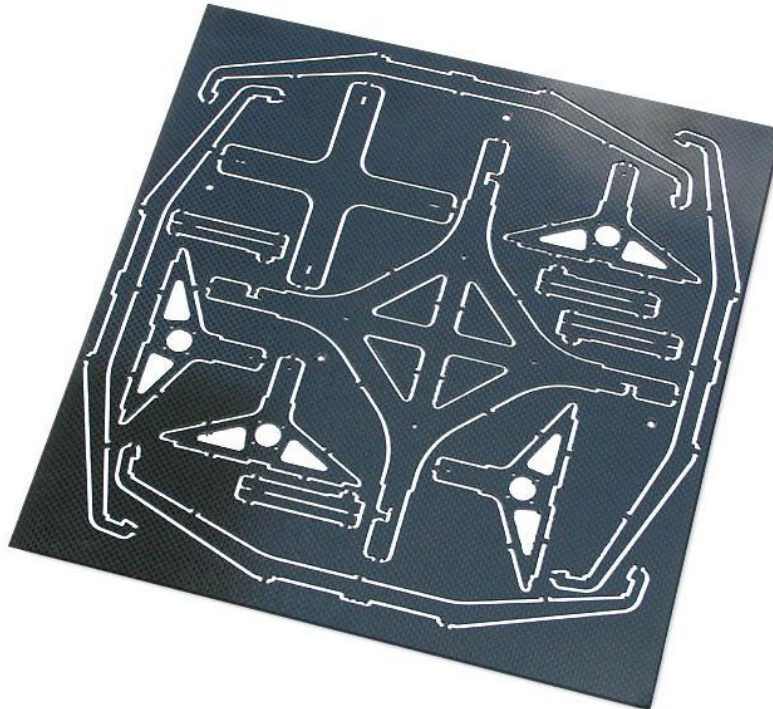
Figure 5. An example of "cookie cutting" a pattern in a sheet of carbon fiber. In this instance, more than half of the area will be thrown away [8] .
