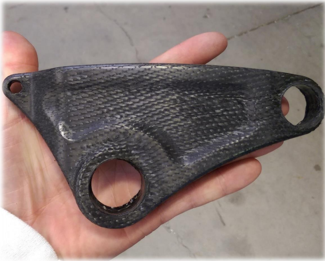
Figure 40. Second iteration of the left rocker arm, outer side showing improved finish and shape over first iteration.
