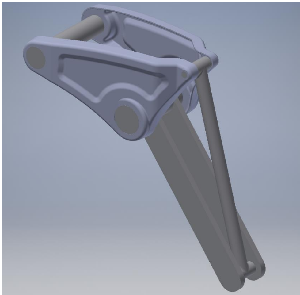
Figure 27. Rocker arm assembly geometry designed for FEA to remove the degree of freedom present in a single rocker arm analysis while preserving the dynamics present in the real system.
