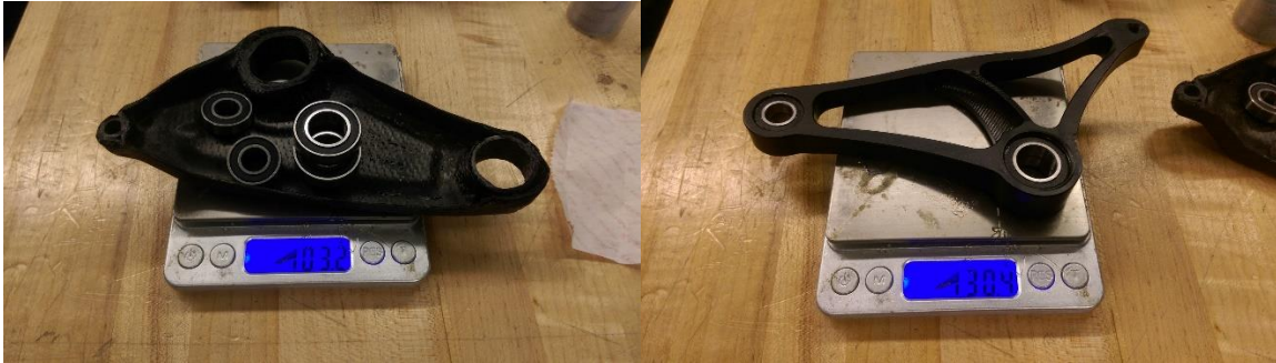
Figure 53. 1 st Iteration carbon rocker weighing in at 103.2g (Left) Aluminum rocker weighing in at 130.4g (Right)
