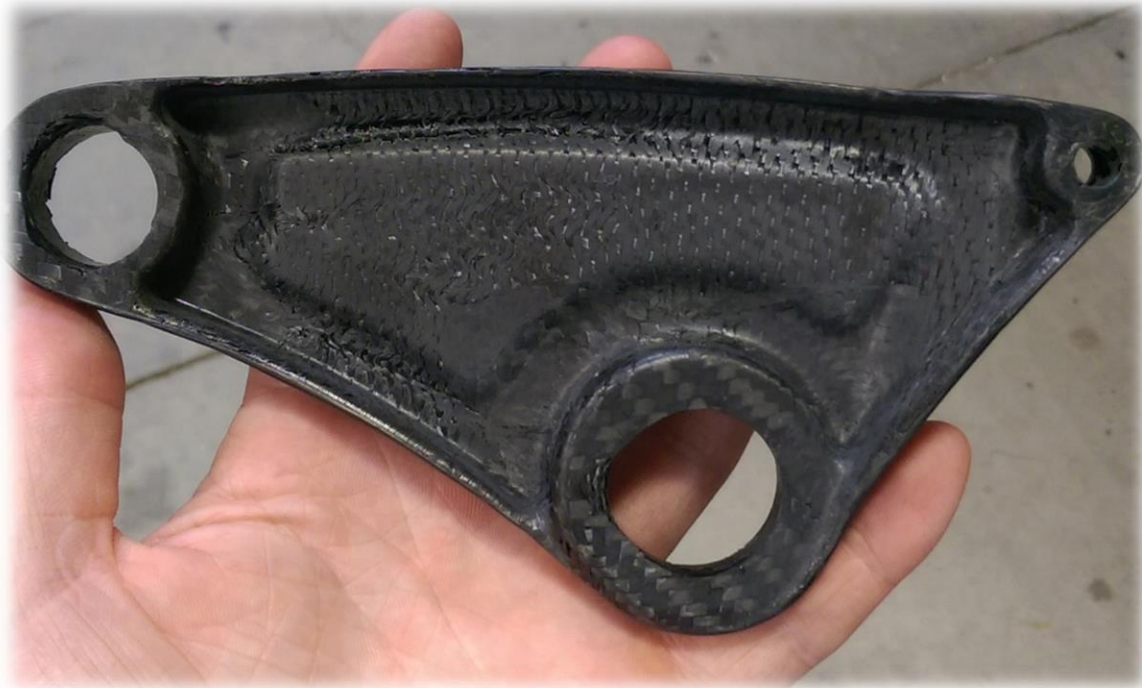
Figure 41. Back side of second iteration of second rocker arm showing improved bearing areas where additional chopped fiber was used. Mold still appeared dry, and needing more resin content.
