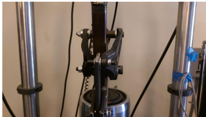
Figure 52. Showing both the carbon and aluminum rocker mounted to the test jig for manufacturing.
