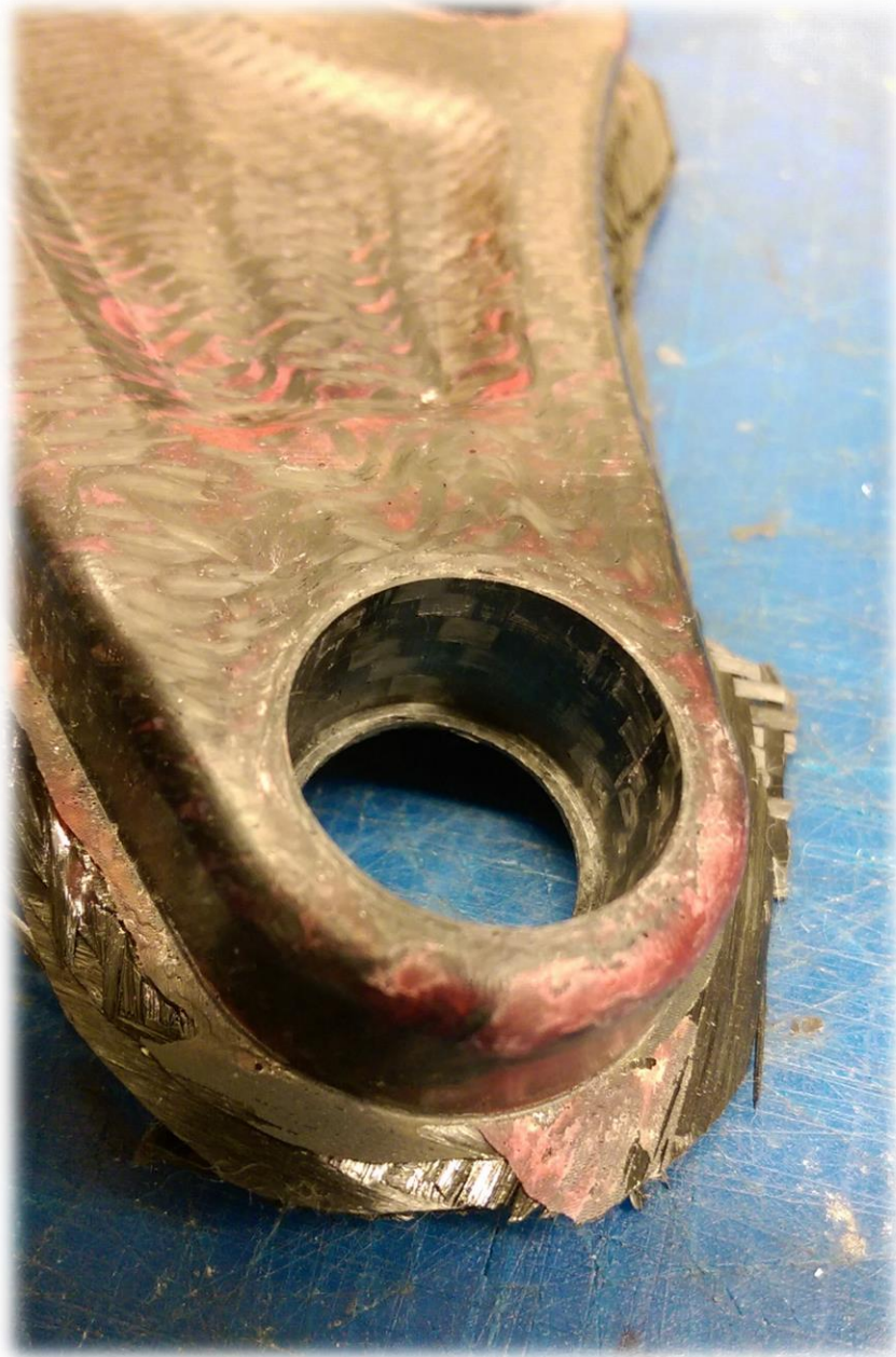
Figure 43. Showing successful transfer of bearing rest from inserts into carbon mold of third iteration, a point of interest which was not obtained in previous molds. In addition, pink areas are areas where adhesive film tape was flashed and filled voids within the mold.
