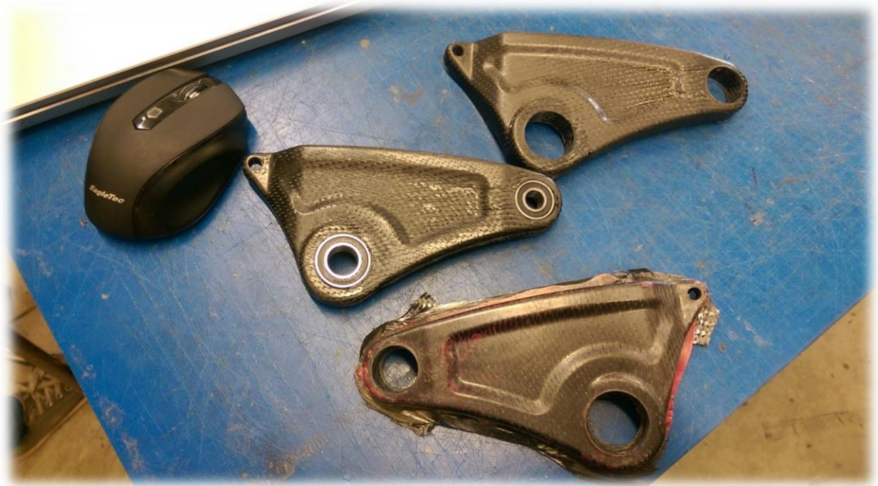
Figure 45. Showing all three iterations of the rocker arm. Top is the first iteration, middle is the second, and bottom is the final right-side iteration. Drastic improvement in shape, surface finish and form can be seen between these rockers.
