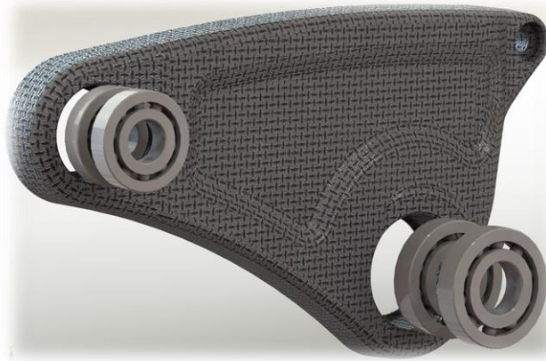
Figure 48. Bearing installation into rocker arm.
