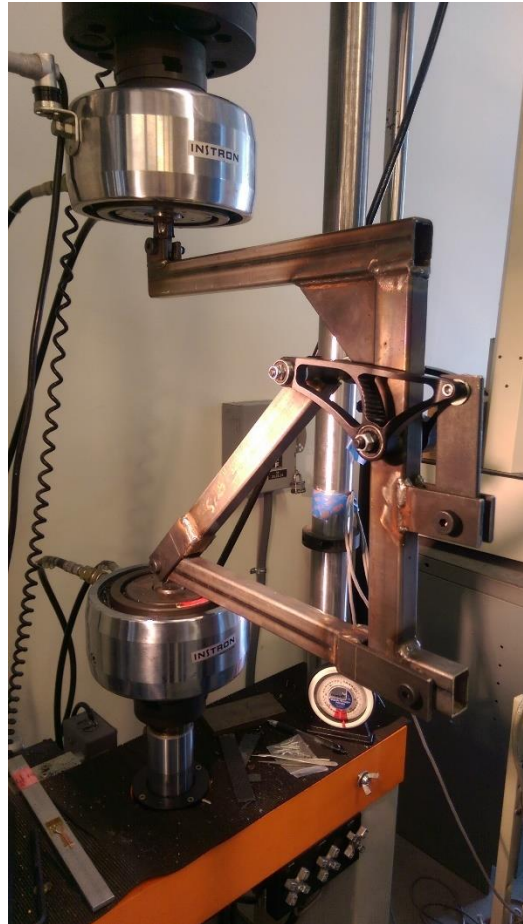
Figure 50. Test jig after grip rotation, being installed into the Instron for testing.
