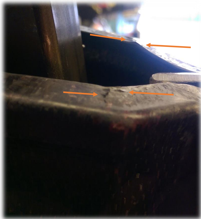
Figure 55. Localized buckling seen on both rockers during testing of rockers for maximum strength.
