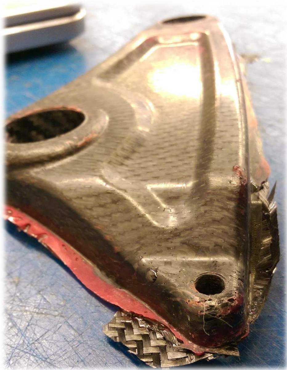
Figure 44. Third iteration of rocker showing excess film tape flashing, but drastic improvement in surface finish and part form due to addition of layer of film tape into layup. Small voids can still be seen at the edges of the front bearing region where it is difficult to pack chopped fiber.
