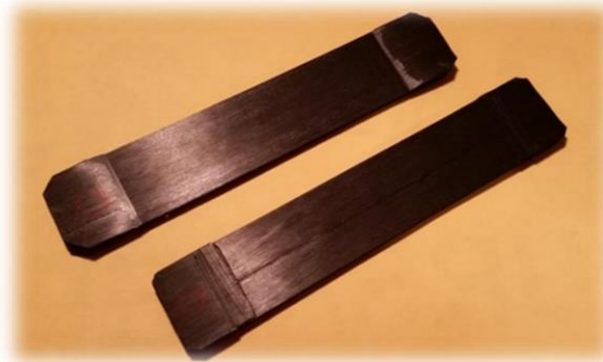
Figure 3. Example of initial tensile specimens created by Corinne Warnock during her research [6]
