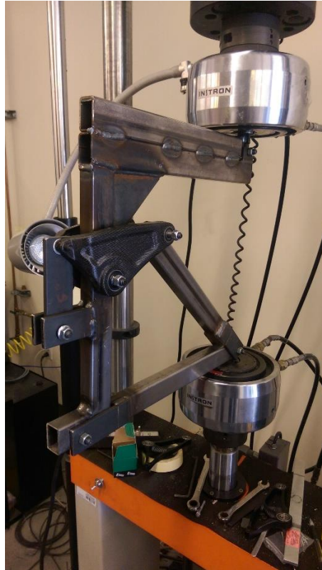
Figure 51. Test jig with welded support on upper load bearing member.
