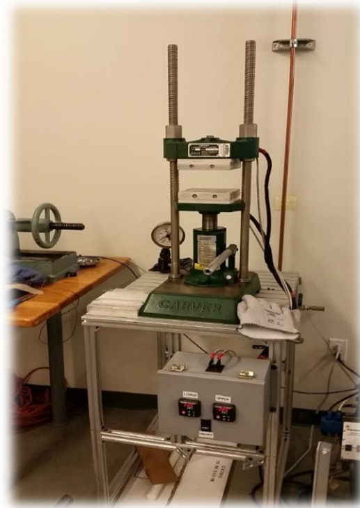
Figure 7. The Carver Model C heated laboratory press located in the composites lab of Engineering IV.
