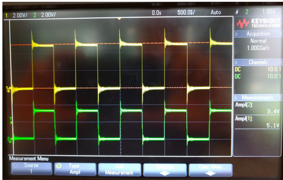
Figure 8.8: TXB0106 level shifter propagating signals from one voltage domain to the other
