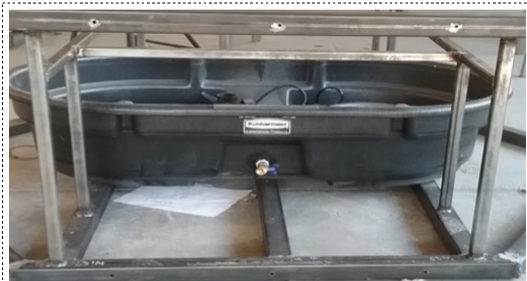
Figure 57: Drain assembly installed in reservoir tank.
