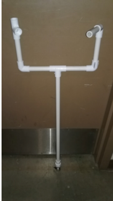
Figure 25: Prototype for the interchangeable water pipes feature
