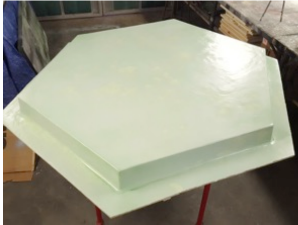
Figure 53: Basin mold with after the final layer of PVA mold release was applied.
