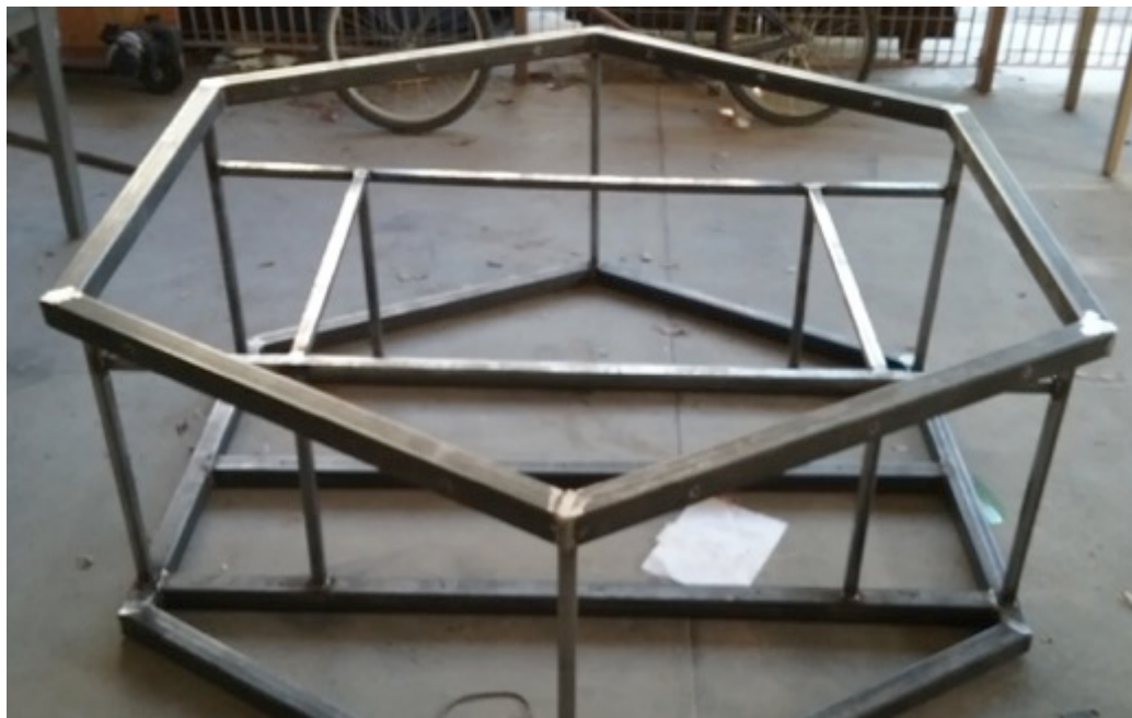
Figure 55: The completed frame prior to Rust-Oleum paint application.
