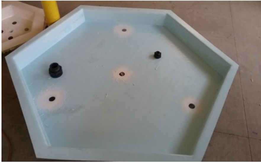
Figure 59: Holes drilled in fiberglass basin to test fit bulkhead fittings.
