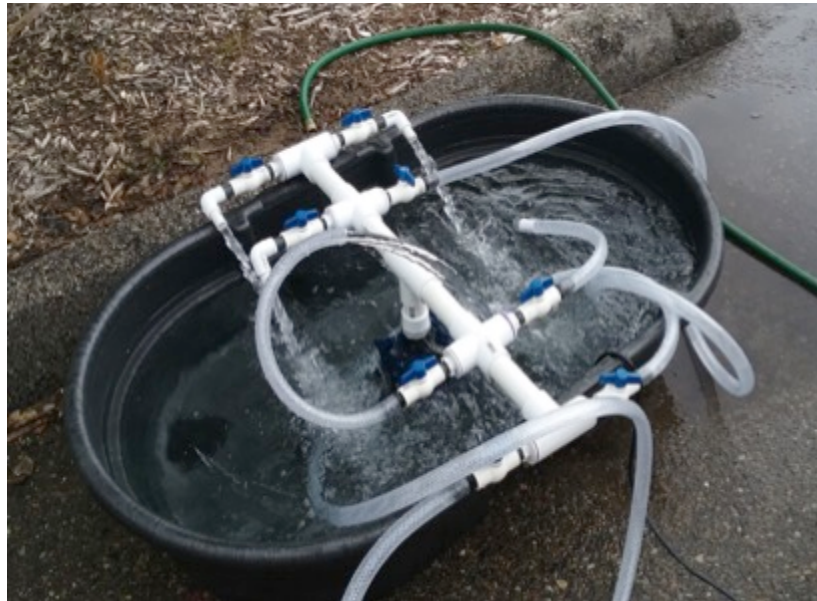
Figure 58: Rigid supply fixture connected to pump shown during operation.
