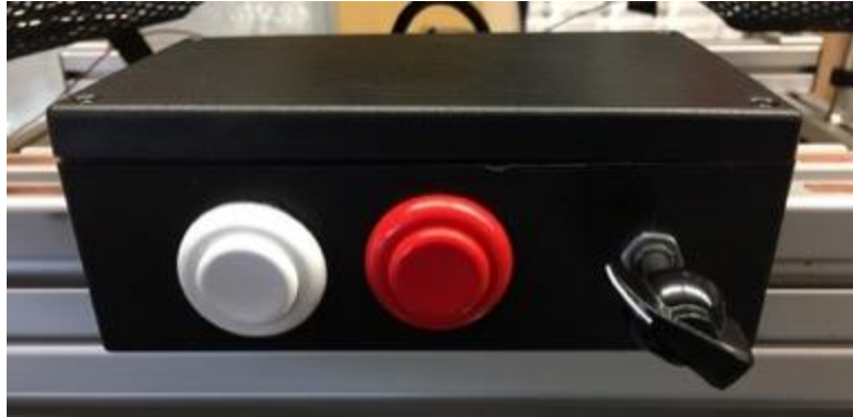
Figure 44. Implemented control panel inputs.
