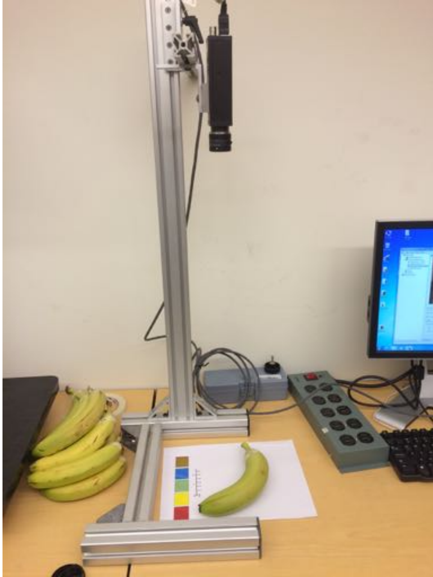
Figure 9: Sony computer vision camera set-up.
