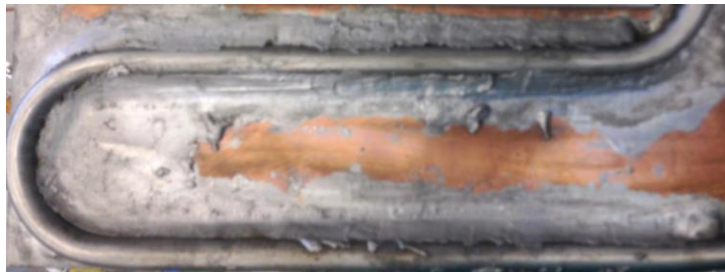
Figure 40. Uneven Brazing of the Pipes to the Platen
