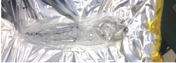
Figure 49. Large blanket test, burnt blanket
