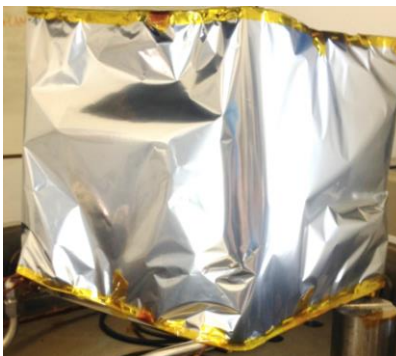
Figure 29. MLI Over the Shroud to Insulate the Copper.
