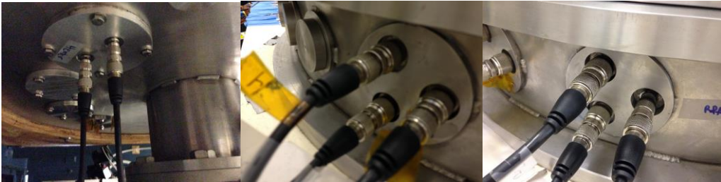
Under the chamber, and two feed throughs on the side of the chamber all need to be plugged in
