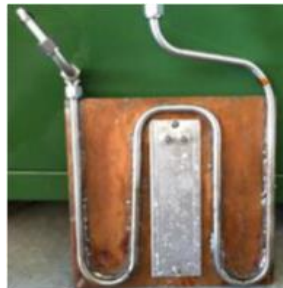
Figure 9. Platen and Piping
