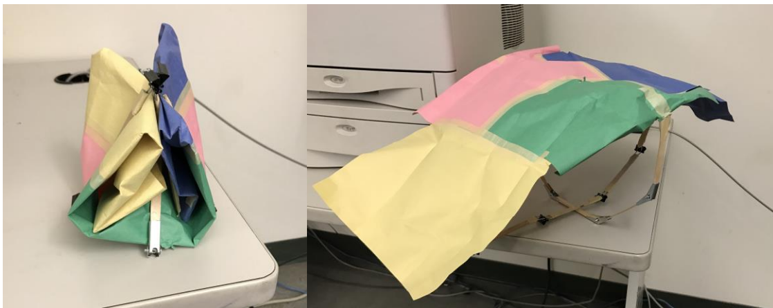
Figure 13. Hinged Boom Concept Model Folded and Deployed.
