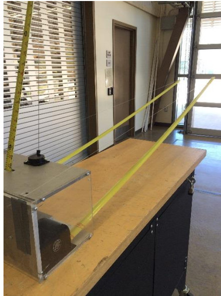
Figure 43. Tape measure booms used for vertical and horizontal deployment.
