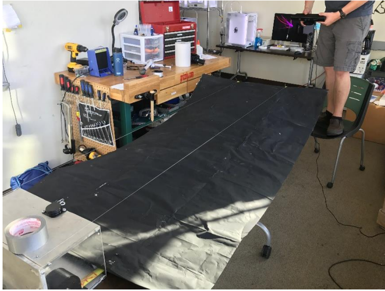
Figure 76. 3-D scanning the reflector (spray painted black) to assess shape.
