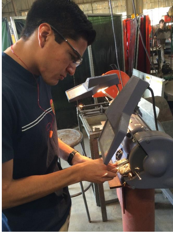
Figure 57. Grinding of the main shaft.
