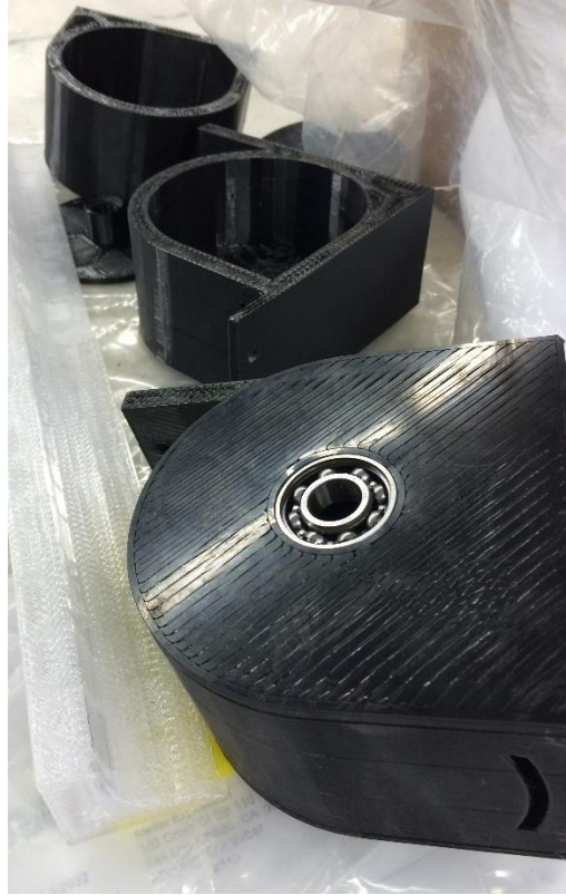
Figure 51. 3D printed deployer housings
