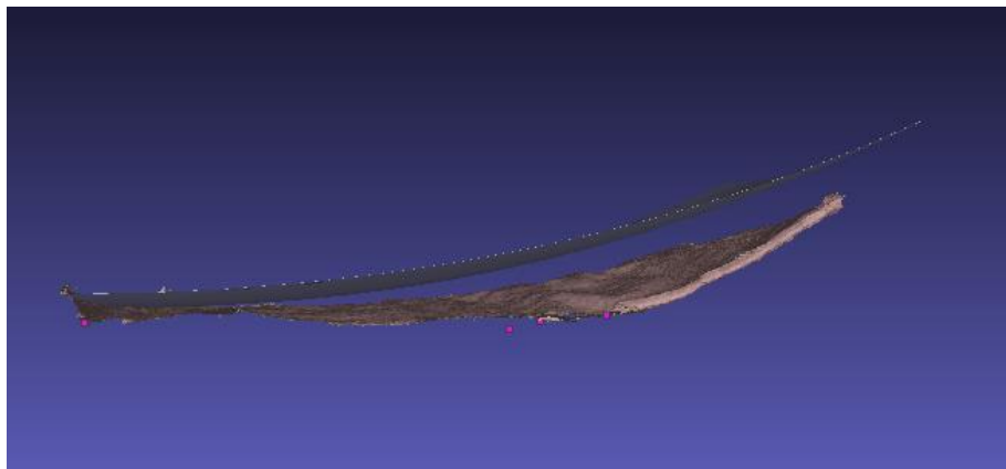
Figure 77. Ideal Parabolic Reflector overlaid with the 3D scanned reflector.
