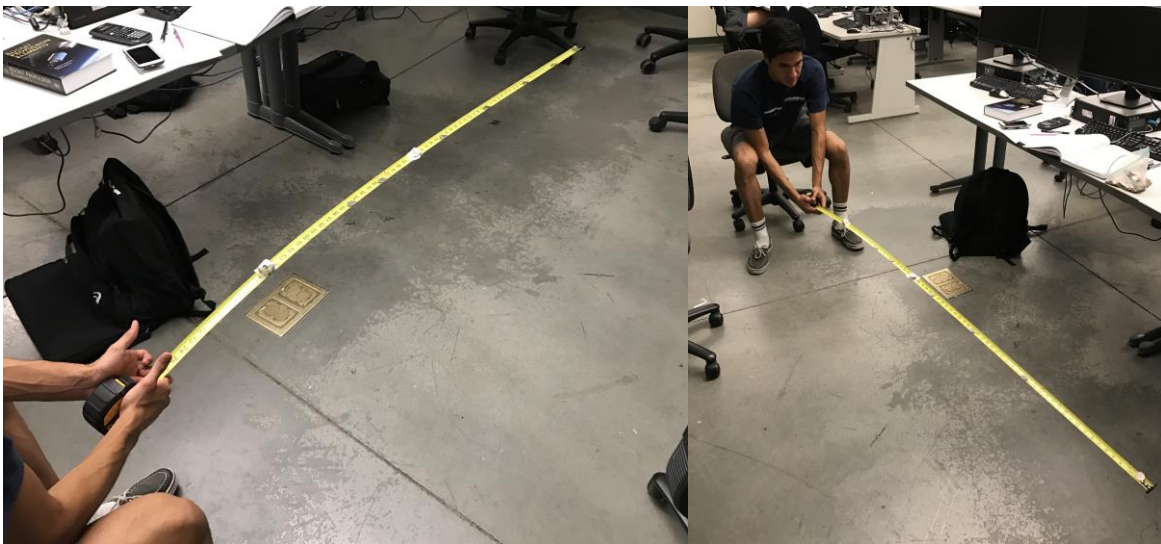
Figure 37. Static Test of Actual Tape Measure Deflection Using Coins as Distributed Load.
