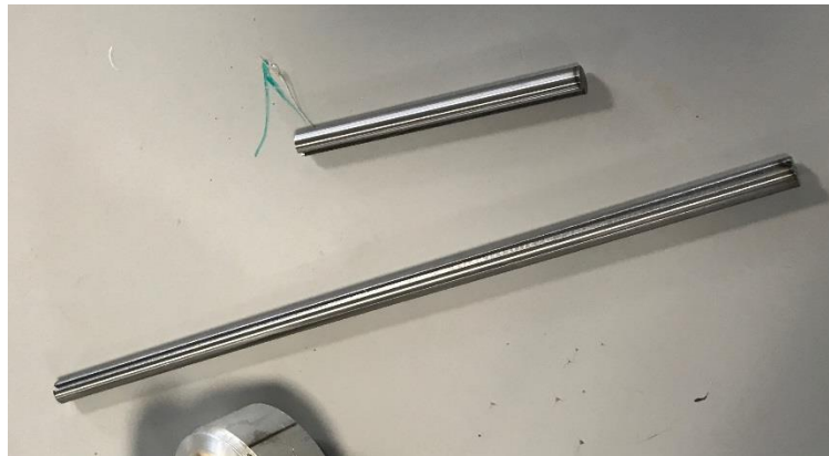
Figure 58. Completed main and feed shaft.
