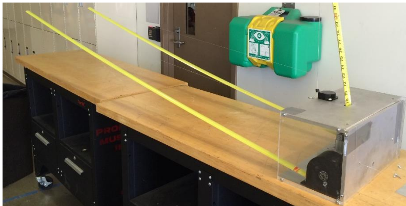
Figure 68. Fully extended deployer assembly with acrylic plexiglass side walls and tape measure material booms.
