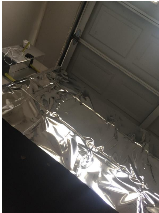
Figure 45. Assembled Mylar reflector.
