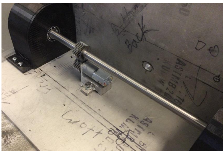
Figure 70. Power transmission to reflector deployers.
