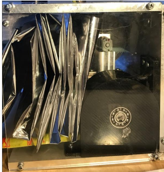
Figure 75. Side view of folded Mylar reflector stored in housing.
