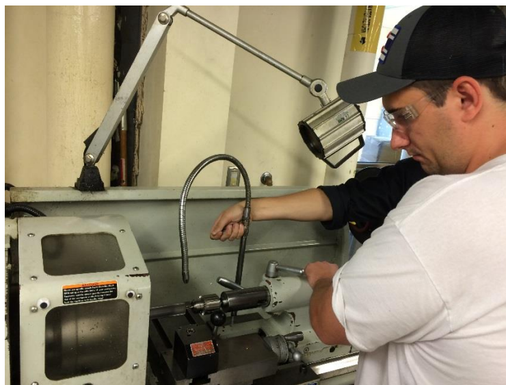
Figure 60. Using lathe to drill concentric 12 mm hole into gear shaft.
