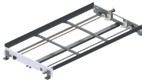
Figure 4-26. X-Axis Power Screw Actuation Assembly
