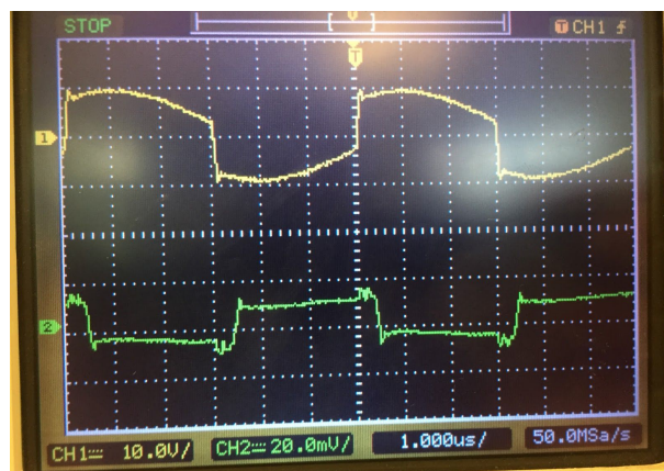
Figure 16: Relay Coil and Transmitter coil Voltages out-of-phase
