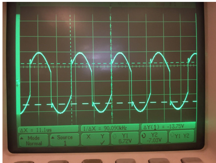
Figure 6: Voltage Across Primary Coil When Powered With Secondary and No Smartphone
