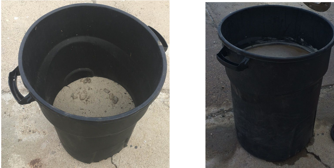
Figure 12. Testing tank (left) sand layer (right) with water.
