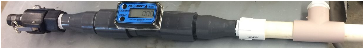
Figure 24. Sensor connection assembly, which contains the flowmeter and the pressure gauge (not shown).
