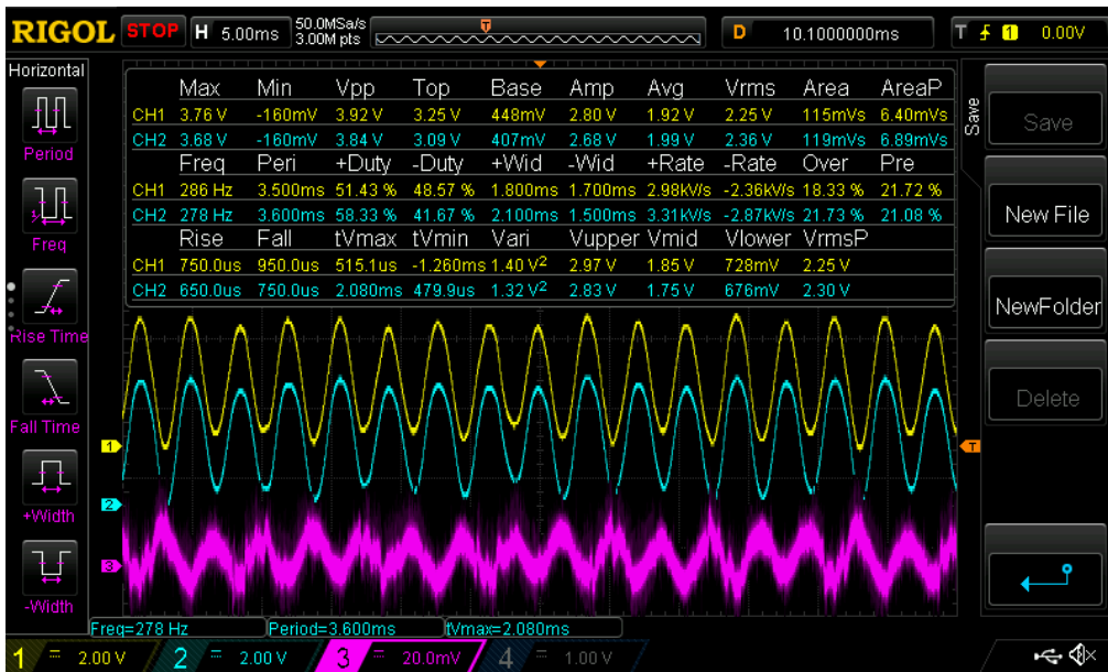
Figure 4.61: Outputs of left (yellow) and right (blue) amplifiers/filters with 15000 gain and a 20 mV, 370 Hz, sinusoidal signal input (purple) which was passed through a 1/75 voltage divider after applying foil box and noise reduction rewiring. Note: trying to capture the input signal after being passed through the voltage divider would inject noise into the input, causing the output to be very noisy so the input could only be captured before going through the voltage divider.
