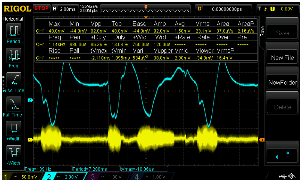
Figure 4.45: Output of left amplifier/filter (yellow) and input (blue) from function generator as a 30 kHz, sinusoidal input signal.
