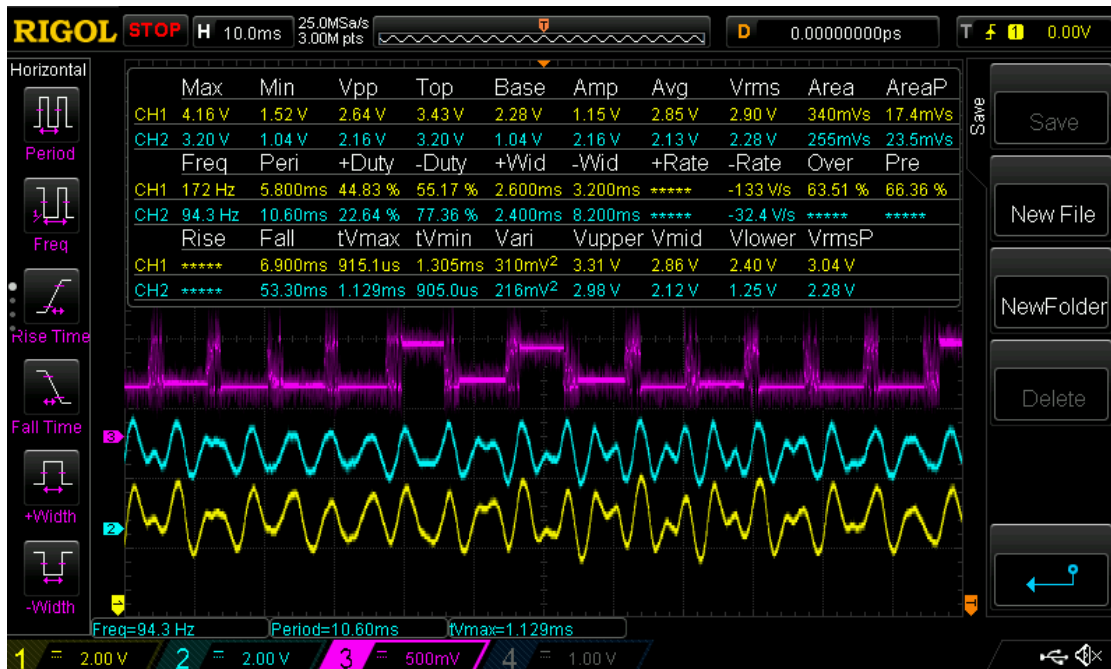
Figure 4.52: Outputs of left (yellow) amplifier/filter, right (blue) amplifier/filter, and reconstructed output of microcontroller (purple), while batteries powered amplifiers/filters.
