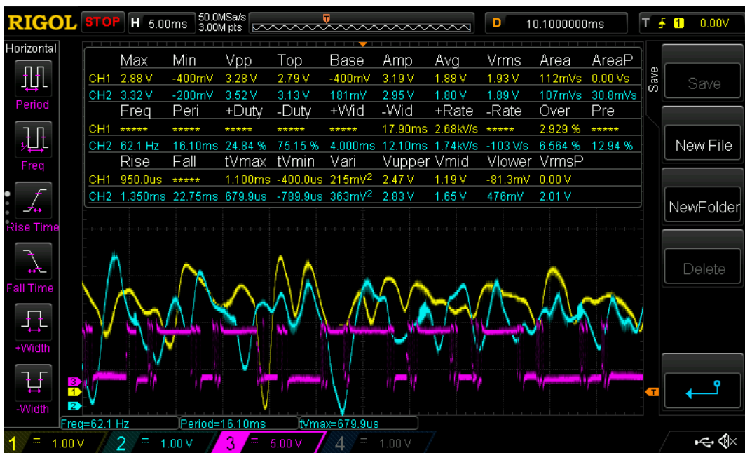
Figure 4.66: Final outputs of left (yellow) and right (blue) amplifiers/filters when receiving inputs from surface electrodes with the “AAA” subvocal signal input “spike” at the beginning of muscle contraction. Wavelet transformed output of microcontroller also shown (purple).
