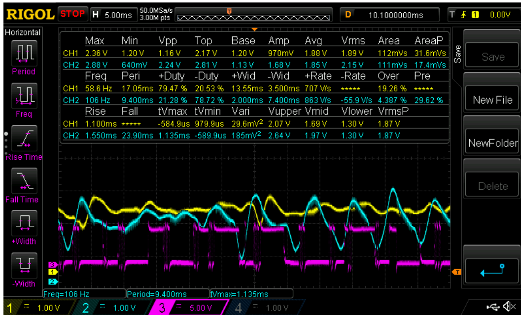
Figure 4.69: Final outputs of left (yellow) and right (blue) amplifiers/filters when receiving inputs from surface electrodes with consistent “IIII” subvocal signal input after initial “spike”. Wavelet transformed output of microcontroller also shown (purple).
