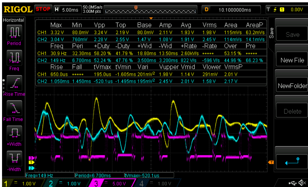
Figure 4.68: Final outputs of left (yellow) and right (blue) amplifiers/filters when receiving inputs from surface electrodes with consistent “EEEE” subvocal signal input after initial “spike”. Wavelet transformed output of microcontroller also shown (purple).
