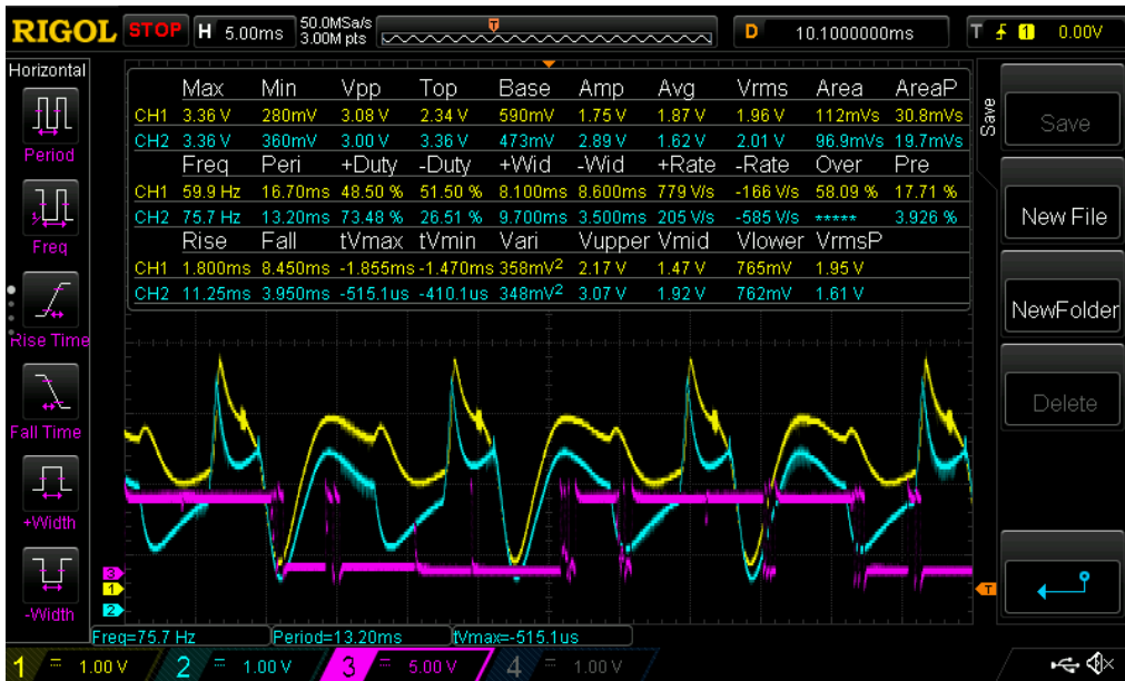
Figure 4.62: Outputs of left (yellow) and right (blue) amplifiers/filters when receiving inputs from surface electrodes without using the user as ground. Wavelet transformed output of microcontroller also shown (purple).
