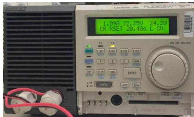
Figure 5-3 PLZ303W electronic load to simulate the load
