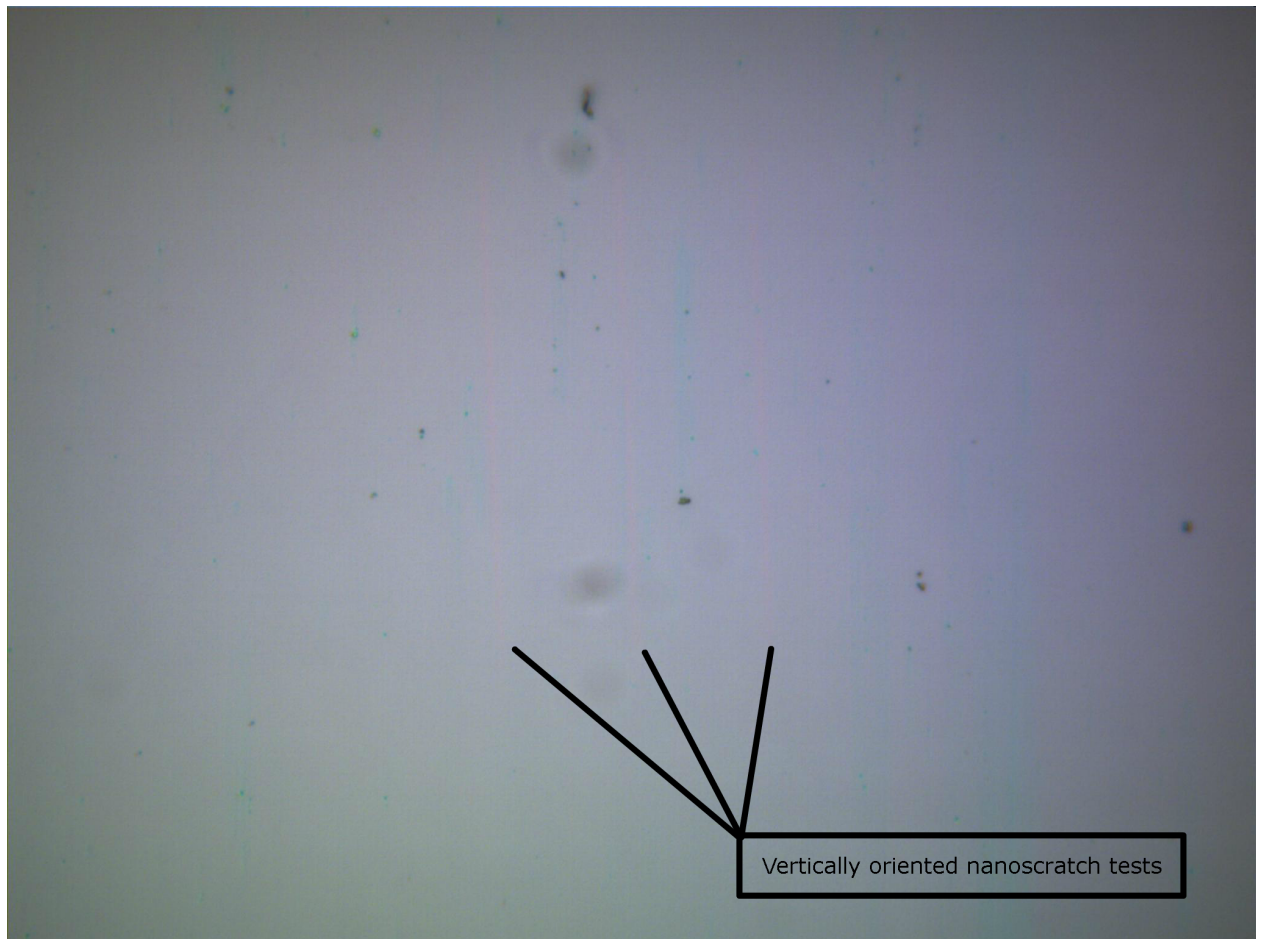
Figure 4.4: An example of a nanoscratch image. There are three vertical scratches in this image, parallel to each other and near the center of the field. They appear as red-orange discolorations, just above each of the black label lines.
