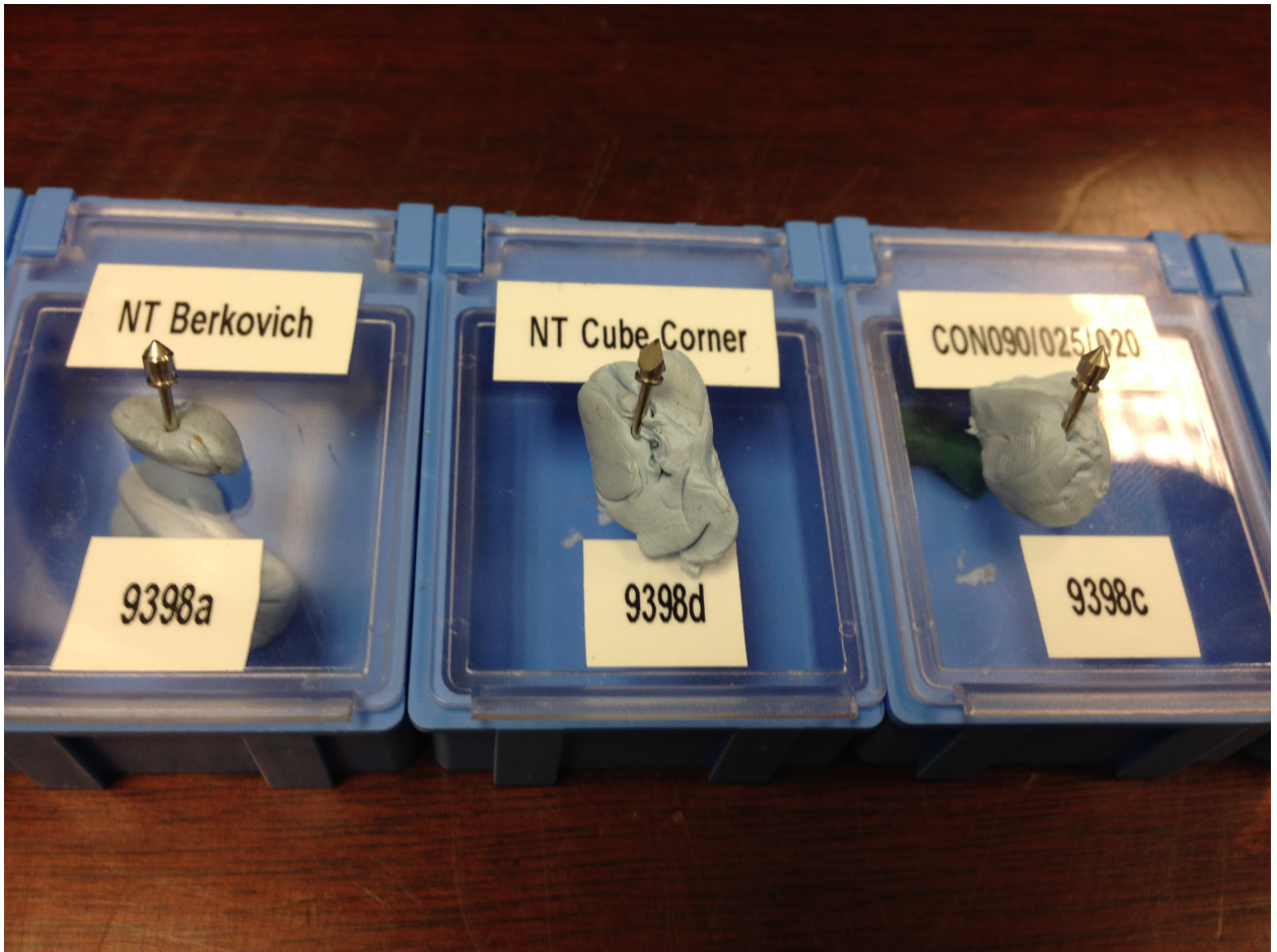
Figure 3.3: The selection of indenter tips used in this study. From left to right: Berkovich, Cube Corner, and Conical.
