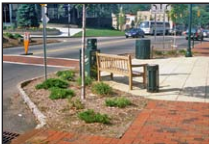
Often associated with “walkable” communities, bulb-outs help slow down traffic in heavy pedestrian environment, and provide area for benches and landscaping.
