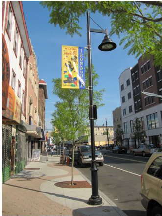
Twenty-five foot downward facing street lights with sheilding to minimize light glare
