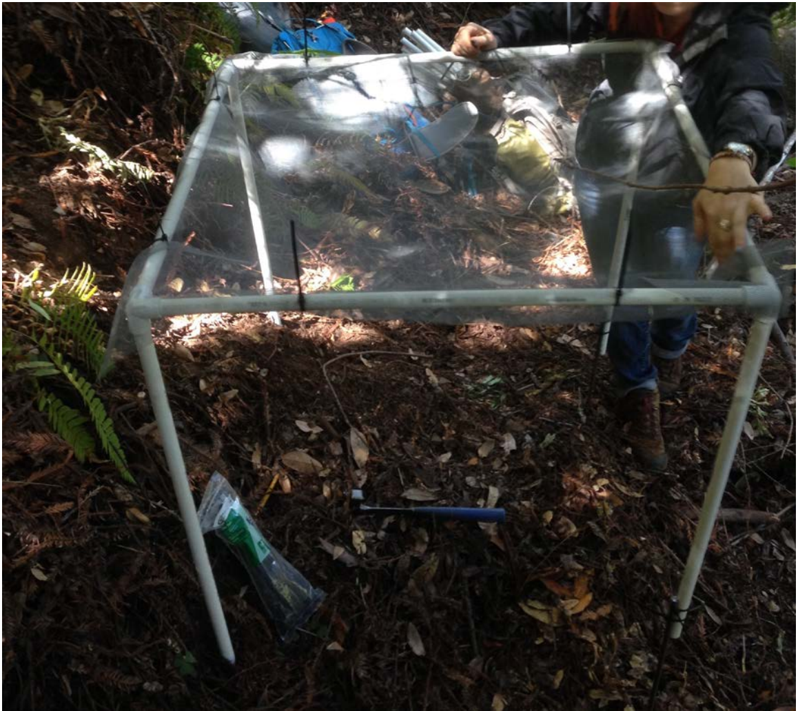
Figure A.23. A constructed seed rain trap. A PVC square was first constructed for the top of the trap, then the legs were attached, then the square of window screen ziptied on with some extra allowed to hang down in order to catch seeds and cones as they fell.
