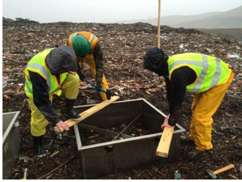
a) Embedment Process of the the Collar
