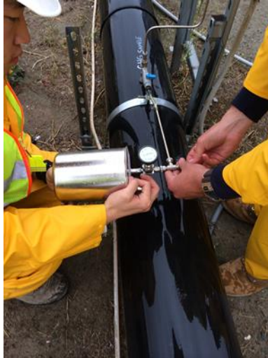
Figure 24 – Photograph of the Sampling Process of the Raw LFG from the Open Flare System
