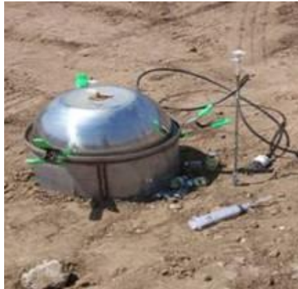
Figure 16- Static Flux Chamber Installed at a California Landfill (Photo by Dr. Jean Bogner)
