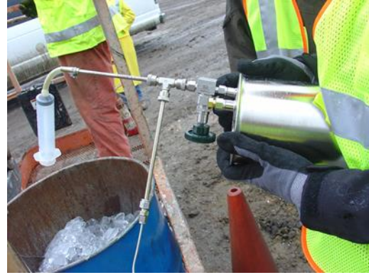
b) Tee Tube Sampling Connection
