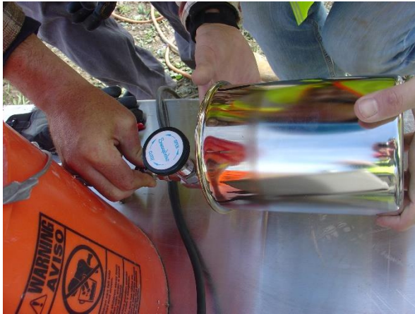
a) Gas being Sampled using 2-L Canister
