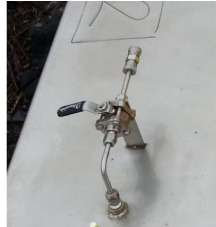
b) Swagelok Gas Sampling Port
