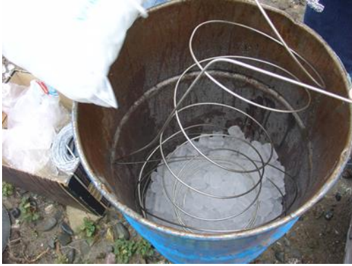
a) Stainless Steel Coil with Ice Bath
