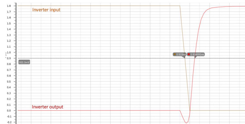
Figure 3.13 CMOS inverter fall-to-rise delay simulation
