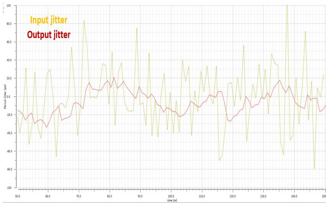
Figure 5.16 Integrator period jitter reduction simulation plot
