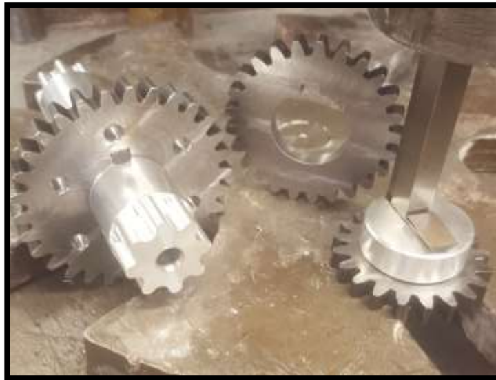
Figure 23 – Push Broach Cutting Keyways into Gears
