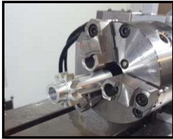
Figure 24 – Test Mid Shaft After Cutting Gear Tooth Profiles
