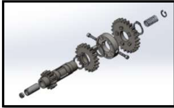
Figure 17 – Exploded Mid Shaft Assembly Schematic
