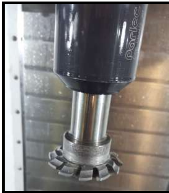
Figure 25 – Arbor Mounted Gear Cutter Used for Mid Shaft
