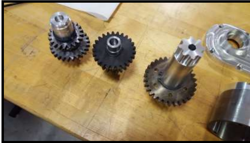
Figure 28 – Three Shaft Assemblies Ready for Installation
