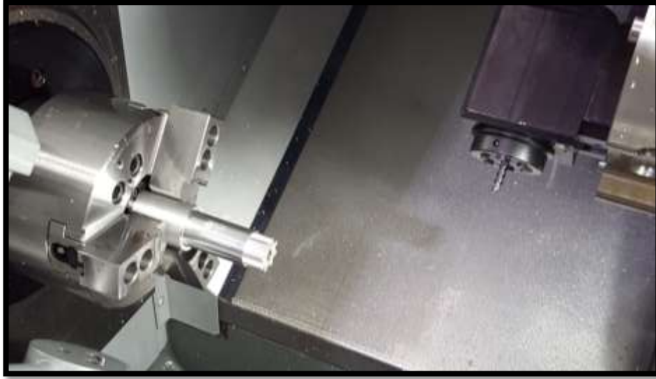
Figure 22 – Testing Radial Live Tooling on Input Shaft
