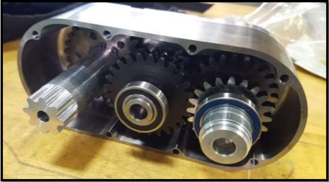
Figure 29 – Three Shafts Installed into Housing
