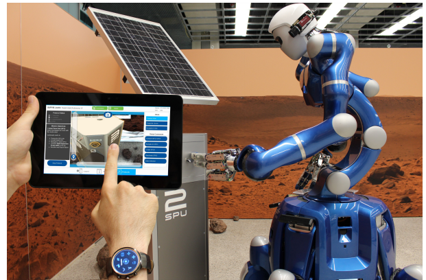
Figure 1. The humanoid robot Rollin' Justin from DLR maintaining a solar panel in a simulated Martian environment. It is commanded via a tablet computer complemented by a smartwatch user interface.
