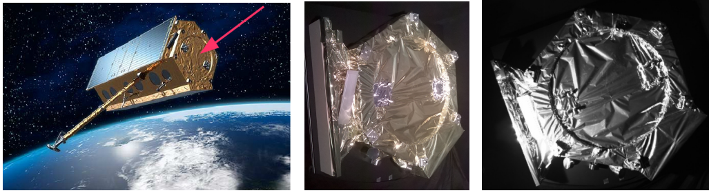
Figure 10. The German Radar satellite TerraSAR-X (left), the full scale mock-up of the rear part of the TerraSAR-X under indoor lighting (middle) and lighting similar to space (right). The arrow indicates the part of the TerraSAR-X satellite used to build the mock-up shown in the middle.
