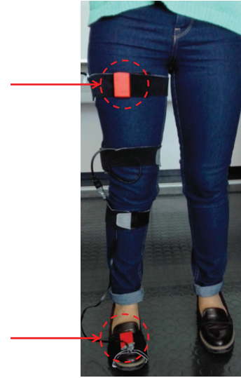
Fig. 5: IMU setup during the experiments. One IMU is placed on the upper thigh. The other IMU is placed on the front part of the foot.
