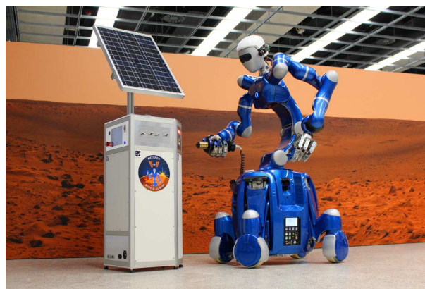
Figure 1. Rollin' Justin maintaining a solar panel in the METERON SUPVIS Justin experiment.
