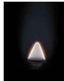
Figure 2: Photography of a conical flame for 50% ( \text{C}_2\text{H}_4 / \text{N}_2\text{O} ) + 50% \text{N}_2 at T_{\text{preheat}} = 473 K, ambient pressure, and an equivalence ratio of \phi = 1.5
