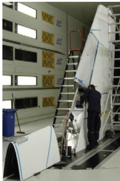
Figure 51: Installation of the HLFC fin on middle section at DNW-LLF wind tunnel [84]
