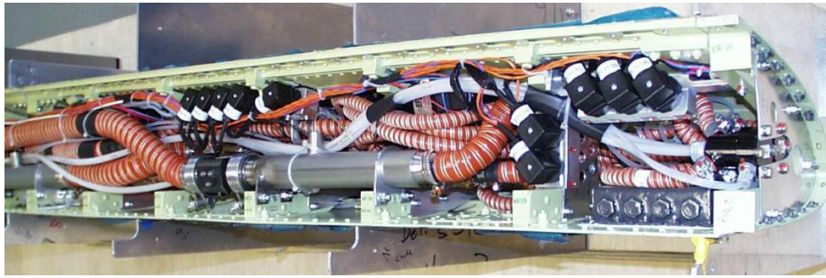
Fig 2. Leading edge of the Do 228 test aircraft equipped for HLFC flight test [83]
