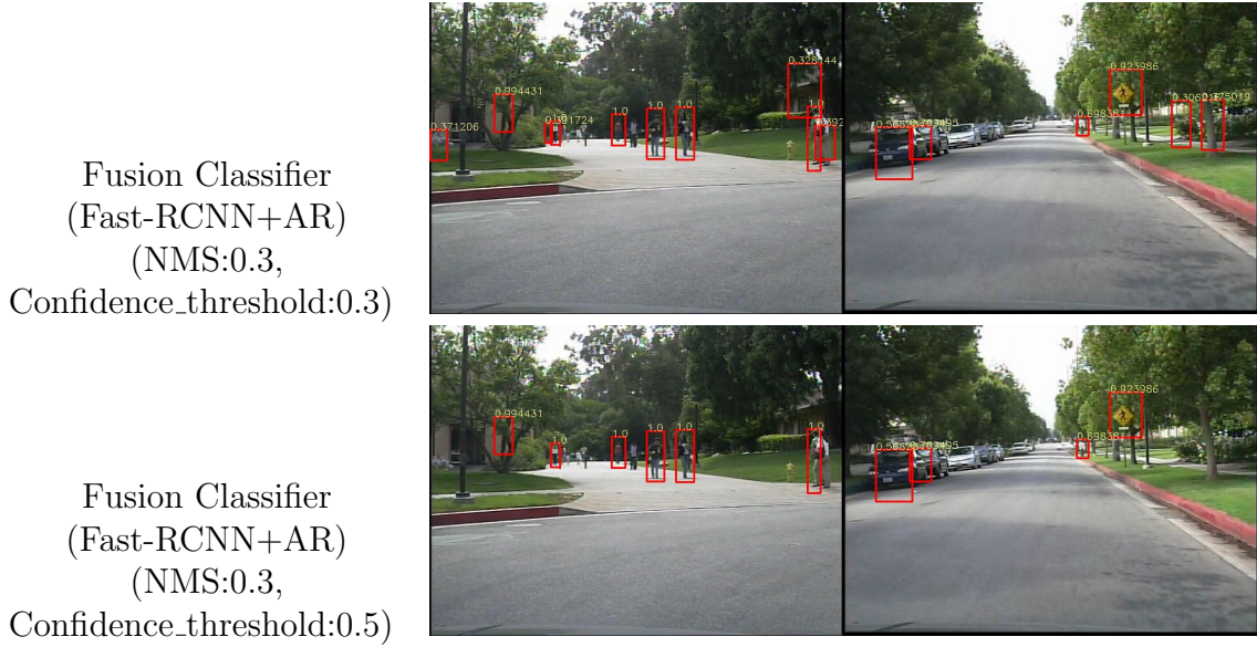
Figure 27: Overview of detection from Fast-RCNN, Context-based(aspect-ratio) classifier and Fusion classifier at different
