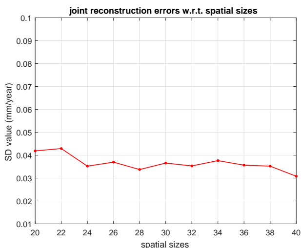
Fig. 3. The plot of the errors of our result w.r.t. different spatial sizes ranging from 20 \times 20 to 40 \times 40 pixels. It is shown that there is no significant difference in the efficiency, as their SDs are all around 4 \times 10^{-2} (mm/year) under the same noise level (SNR=5dB).
