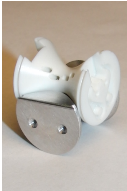
Figure 5.2: Hyperboloid joint of the finger base
