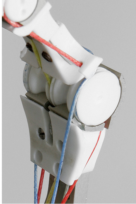
Figure 5.3: Dislocatable hinge joint for the PIP and DIP joints
