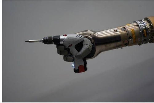
Figure 1.10: Dexhand a space qualifiable hand from DLR
