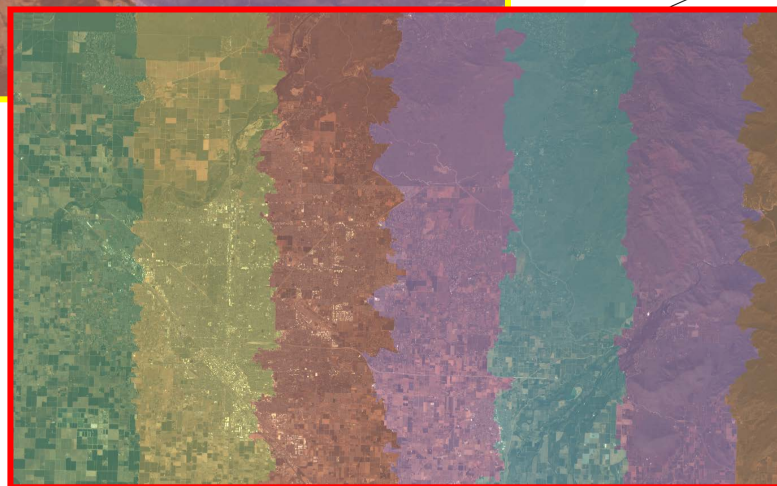
City of Fresno (CA), left image showing gradient based seamlines, right image showing mosaic
