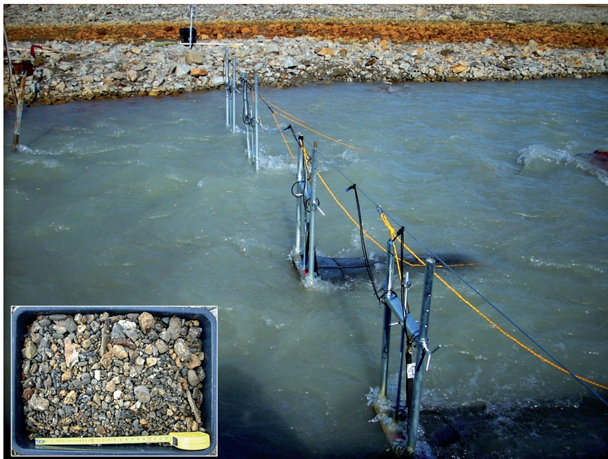
Fig. 3. The set of RBT in the channel cross-profile of the Scott River. Mass of bedload material caught during twenty-four hours in one of measurement sites in the cross-profile of the Scott River
