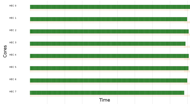
Figure 6.27: Fibonacci Series Sum – HPP Execution Profile from Threadscope – 44 on 8 cores
