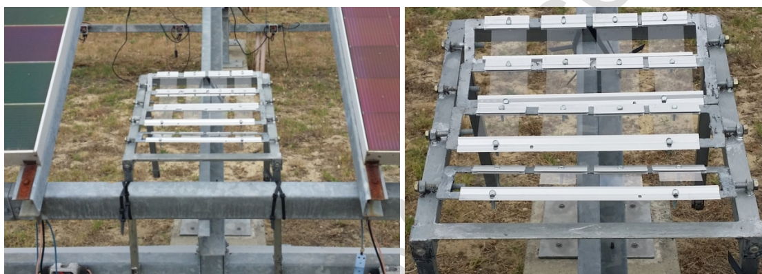
Figure 2. A structure and its close-up appearance that was used to hold glass samples at ROTA
