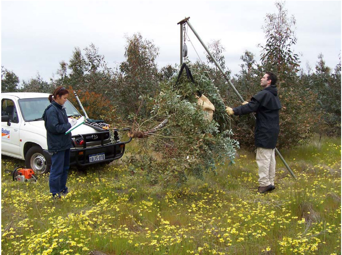
Figure 5.1 Determining component fresh weights with a purpose built bi-pod and weighing scales.
