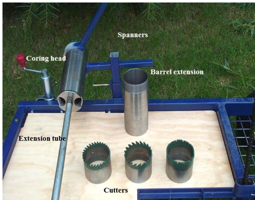
Figure 3.2 Coring head with barrel extension and interchangeable cutters (fine tooth, coarse tooth and diamond matrix).
