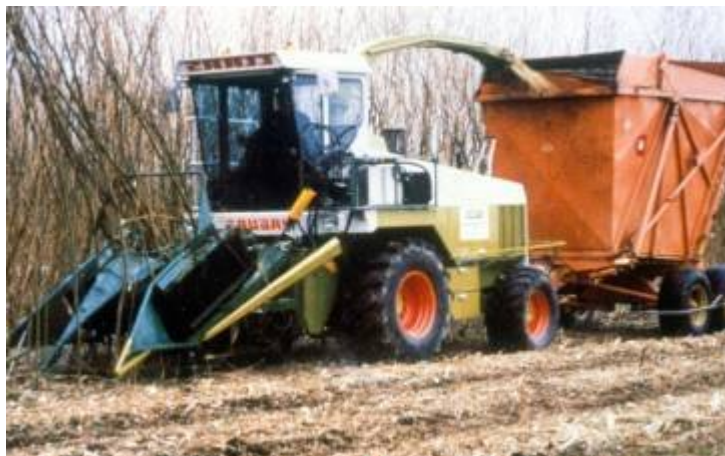
Figure 5-5 Chips being blown into a trailed bin which, when full, is hydraulically lifted and tipped into high sided trucks for transport to store
