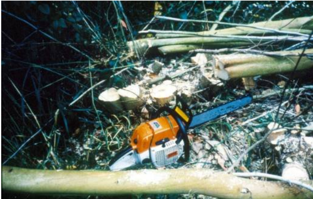
Figure 6-8 Harvesting large or small trees (or in this example, 3 year old coppice Eucalyptus regrowth) can be done manually using a chainsaw with varying cutter bar lengths to suit the tree stem diameter
