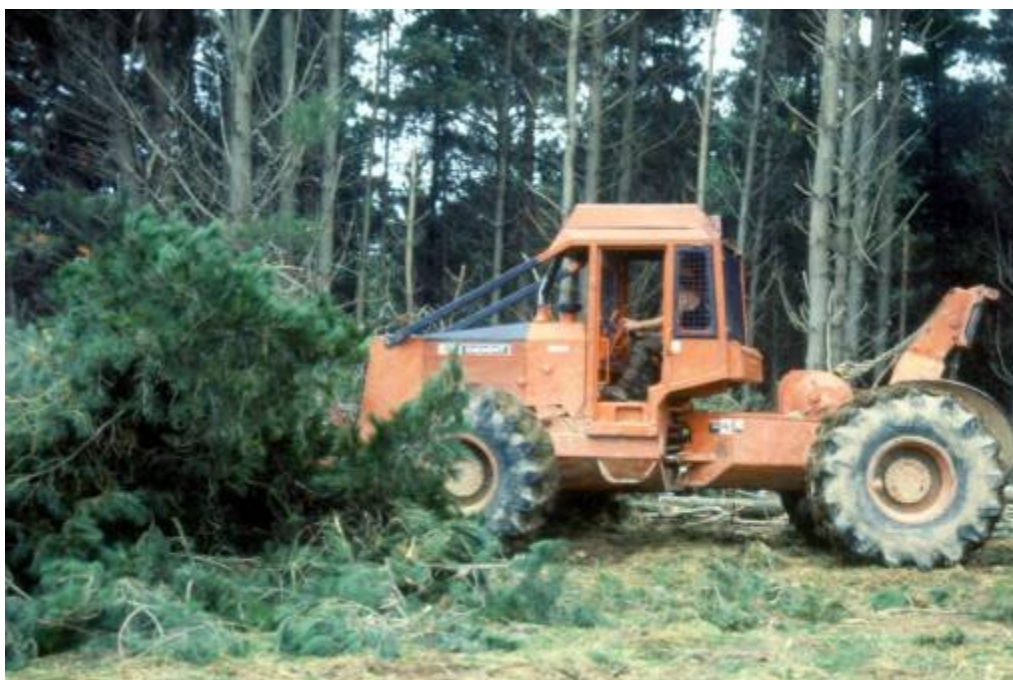
Figure 6-5 Articulated winch skidder working in poorly managed 30 year old P. radiata plantation with a large proportion of material suitable only for bioenergy use
