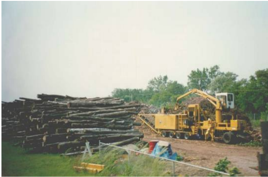
Figure 6-14 Trailer mounted chipper with auxiliary power supply (also available in smaller sizes than shown)
