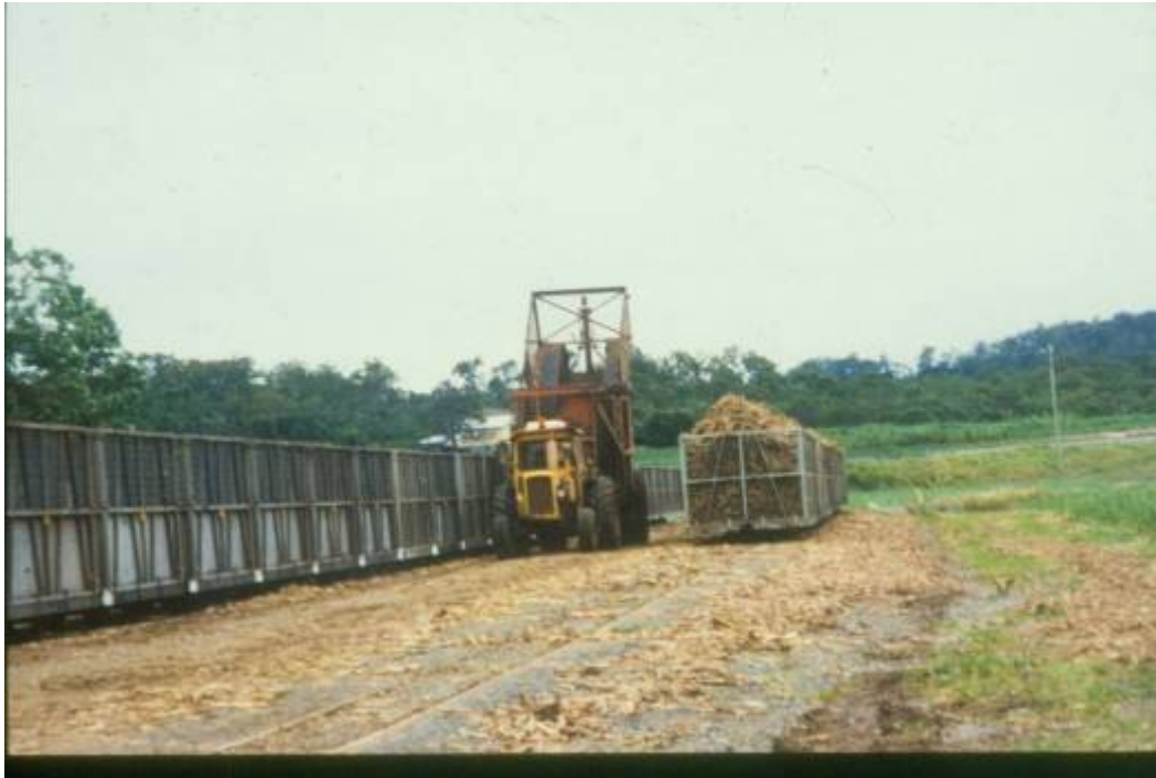
Figure 6-24 Rail bins being filled in the field by the harvester support trailer
