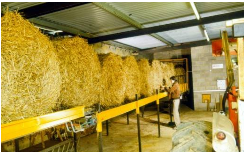
Figure 7-5 Round bales fed into shredder on automatic conveyor to feed straw burner, 24 hours a day and unattended
