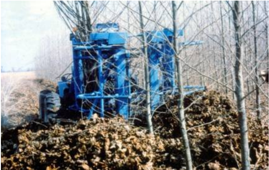
Figure 6-10 Canadian FB7 prototype harvester developed for harvesting SCC poplar trees with stems up to 7 inches (175mm) diameter
