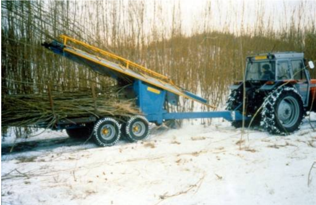
Figure 7-7 Willow stick harvester with collection platform to accumulate load till drop off when full
