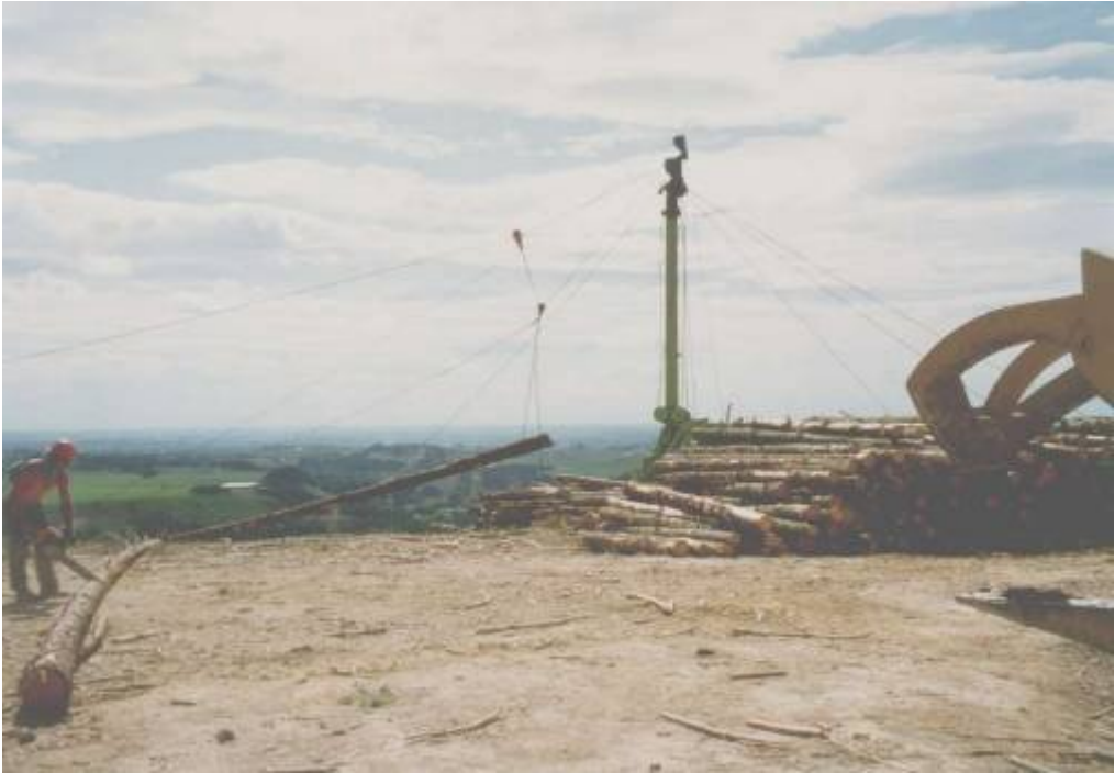
Figure 6-4 Cable hauler extraction of logs in steep terrain up to a landing for removal by transport vehicles after sectioning to length (here shown manually)
