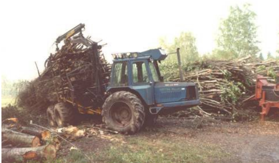
Figure 5-6 Forwarder in Sweden with grapple and trailer for extracting forest arisings and small short cycle crop stems to the landing for chipping
