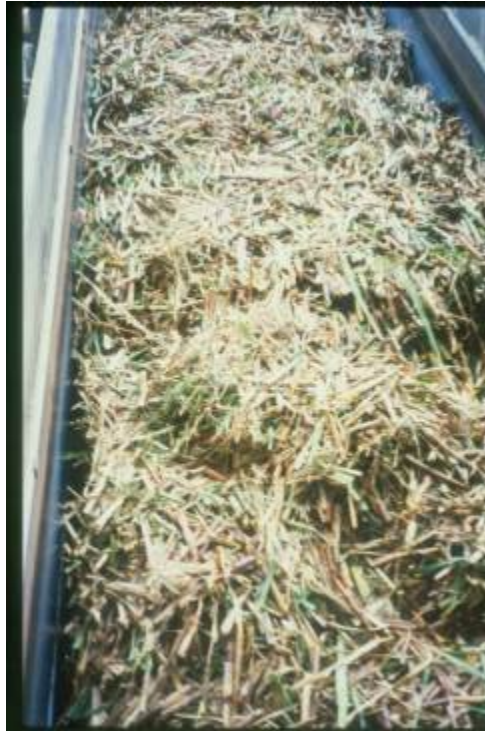
Figure 6-20 Sugar cane billets as delivered from the harvester then fed by belt conveyor into the sugar processing plant
