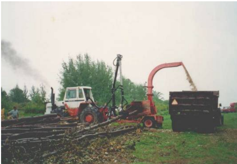
Figure 6-15 Tractor mounted chipper for small-scale applications at 50dt/h and fed by grapple or manually
