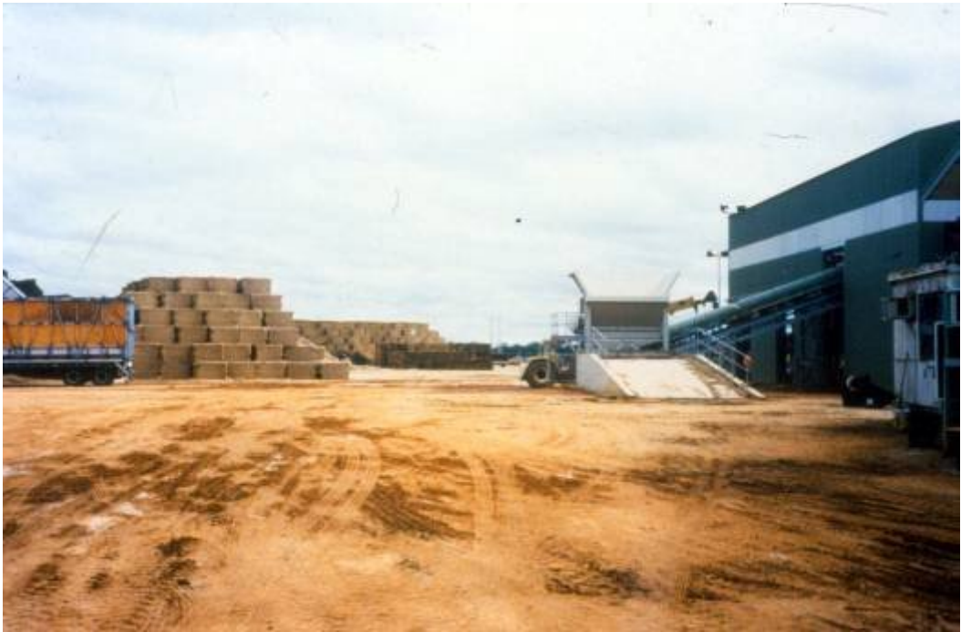
Figure 7-9 Bagasse baled and stored for use in a Queensland sugar processing co-generation plant during the non-cane crushing season
