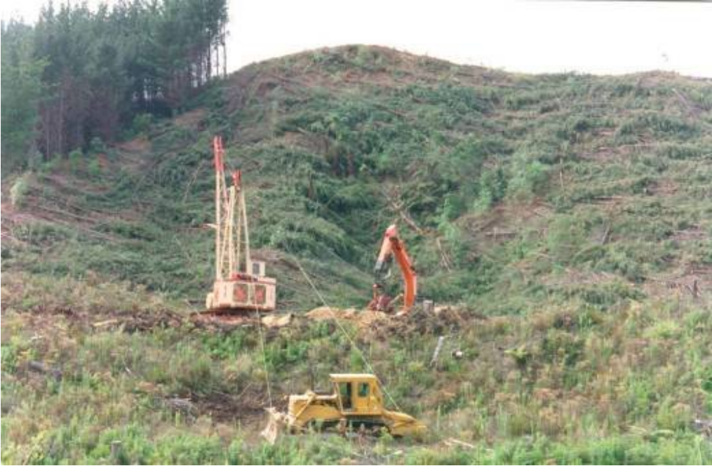
Figure 6-3 Cable hauler tower in P. radiata plantation extracting whole trees down to landing for processing. (Note bulldozer used for anchor only)
