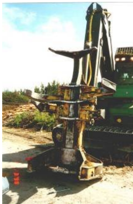
Figure 5-4 One type of design of feller cutting head for single stem harvest of large trees using a hydraulic grab to hold the cut tree during cutting before lying it on to the ground or on to a trailer
