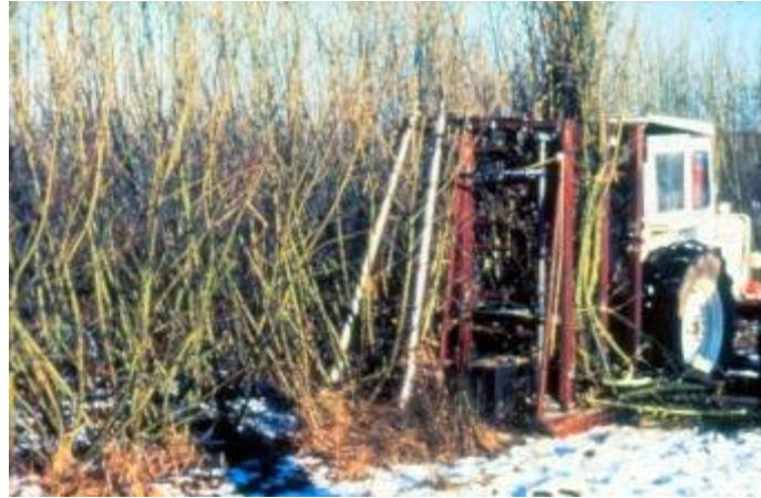
Figure 5-3 Prototype willow harvester from Ireland cutting a double row in one pass and accumulating the sticks into bundles
