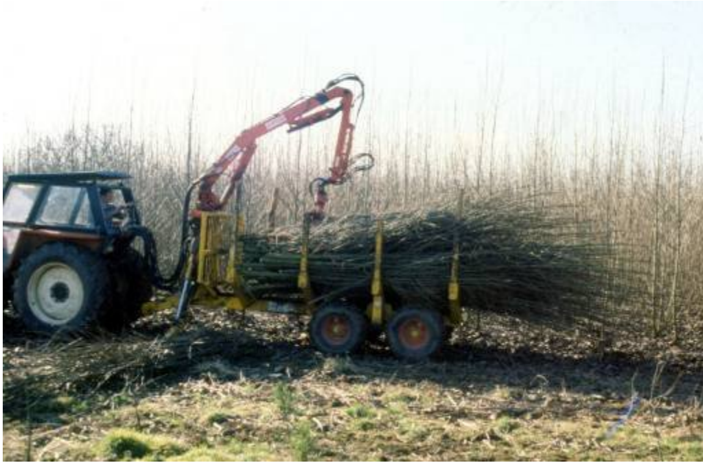
Figure 6-1 Forestry logging trailer with hydraulic loading boom and grapple which can be operated behind a standard agricultural tractor
