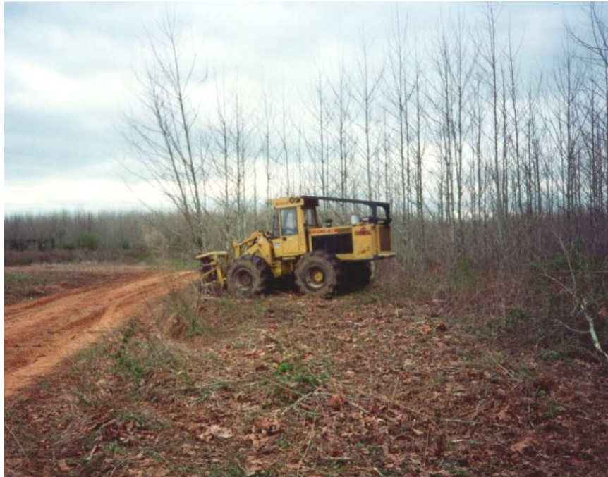
Figure 6-12 Hydroaxe feller buncher harvesting poplars
