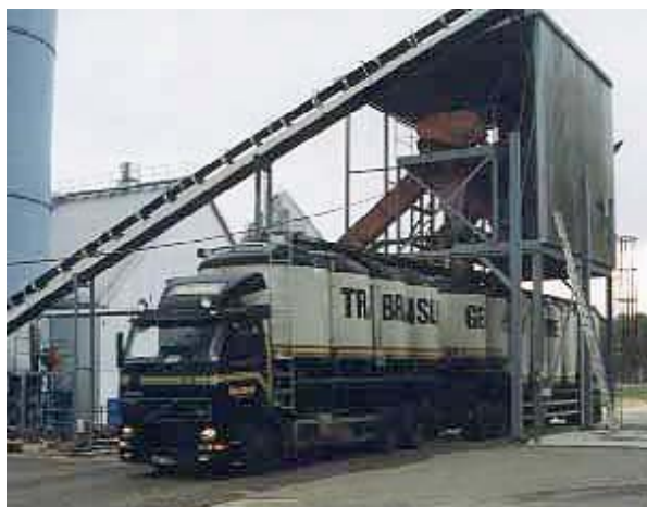
Figure 8-2 Bulk wood pellet tanker in Sweden
