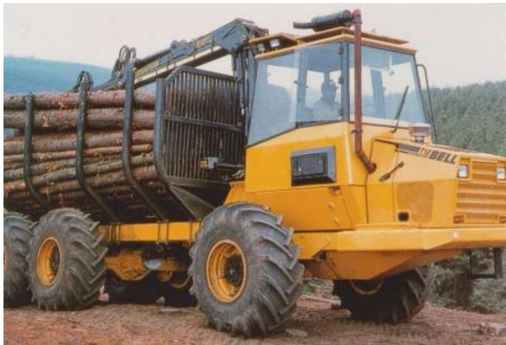
Figure 6-2 Specialist forestry forwarder with articulated chassis
