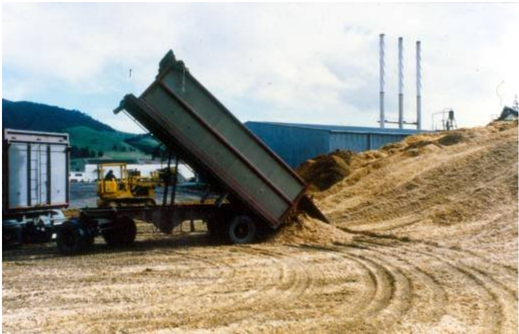
Figure 7-10 Chips being delivered to a Canadian wood-fired power plant by tipping truck
