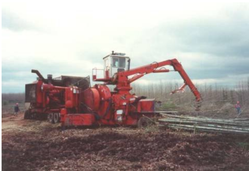
Figure 6-17 Heavy-duty chipper handling SCC poplar at around 30 odt/h with grapple feed
