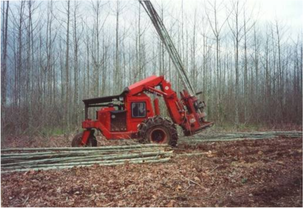
Figure 6-9 Feller-buncher with accumulating head developed for SCC harvesting of poplars in the USA
