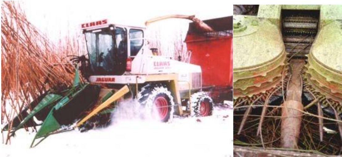
Figure 6-11 The Claas forage harvester with twin disc cutting head developed to harvest SCC willow
