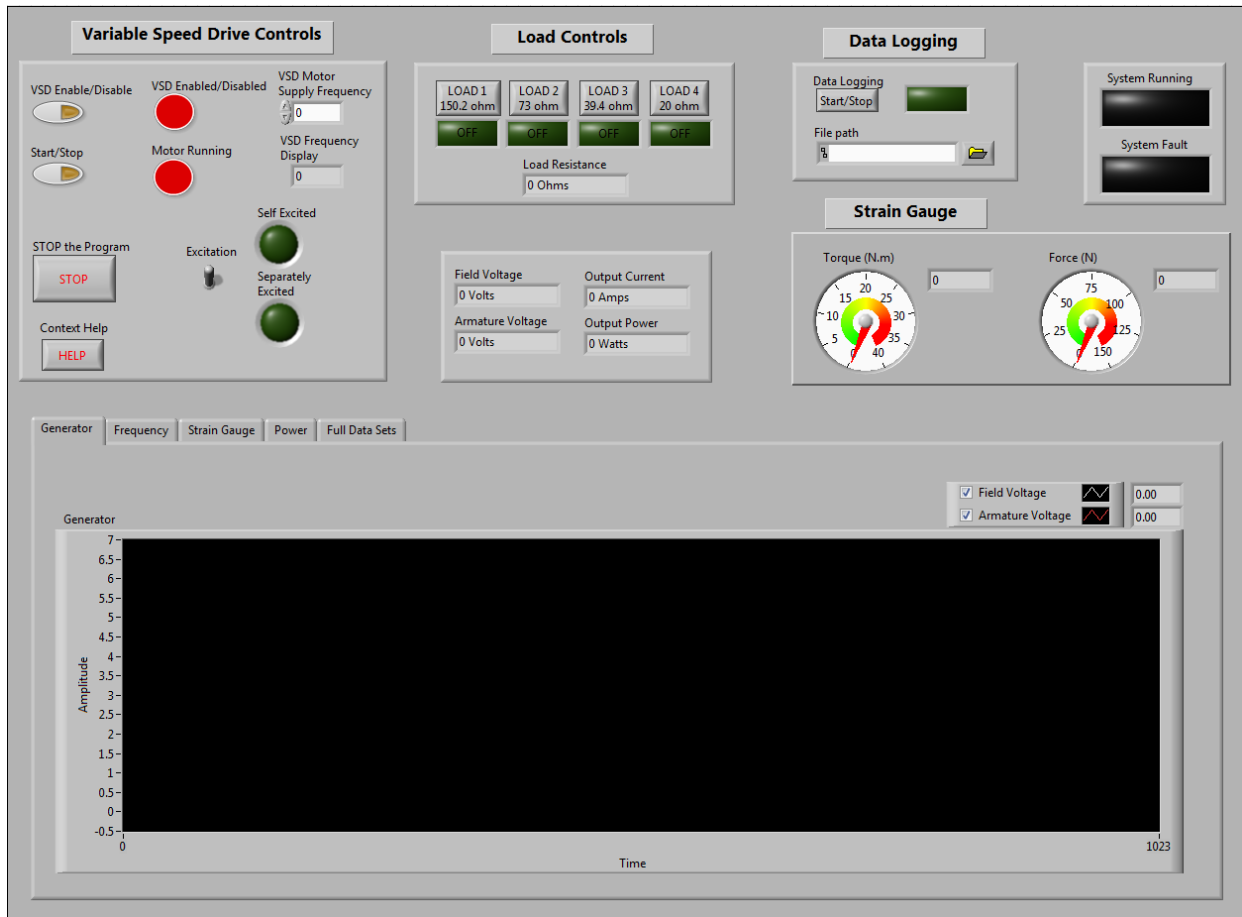
Figure 36: Control and Monitoring Interface
