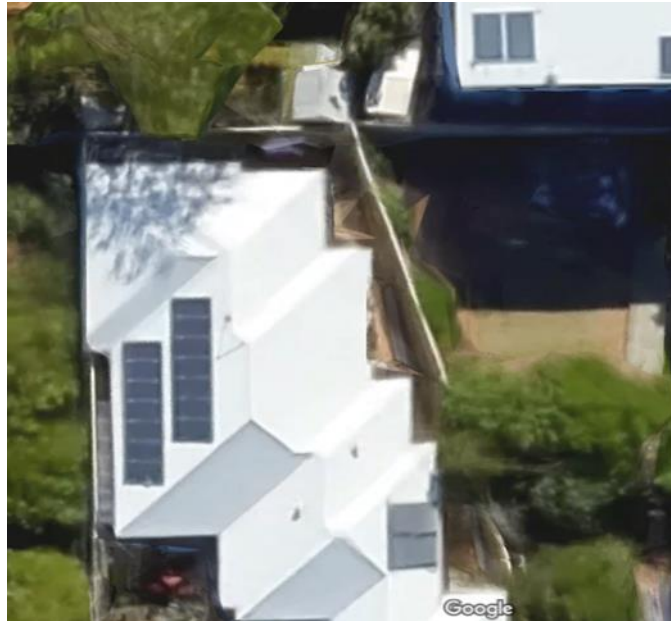
Figure 49: House M with solar collectors positioned so shaded by the tree to the east (source: Google Earth, 6/11/2016)
