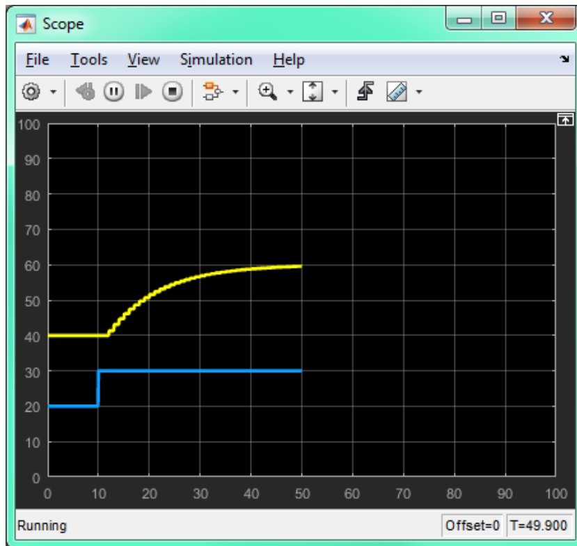
Figure 57: Simulink OPC Testing - First Order System Response at t = 50s
