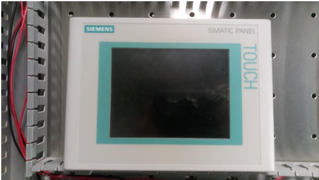
Figure 27 Siemens TP 177B 6" PN/DP HMI Touch Panel
