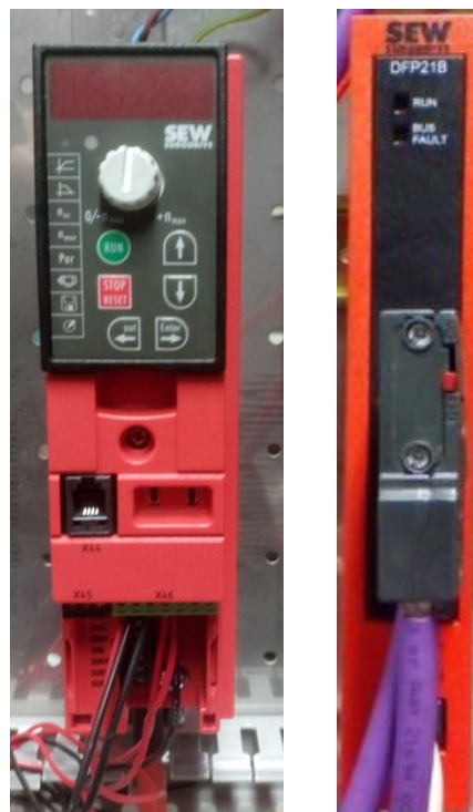
Figure 38 SEW-EURODRIVE MOVITRAC B MC07B0003-2B1-4-00 (single phase) VSD (left) and DFP21B Gateway (right)
