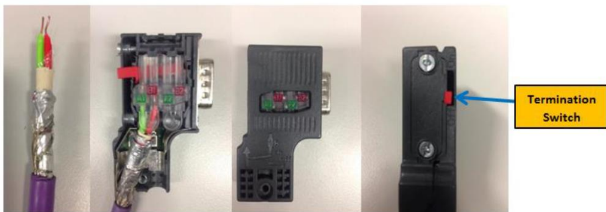
Figure 25 Students learn how to strip and attach Profibus DP cables to Profibus DP connectors and subsequently how to terminate networks using termination switches [29].
