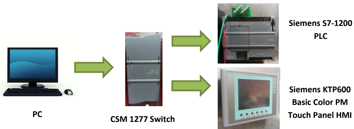
Figure 54 Profinet HMI learning module network structure, based on [61]
