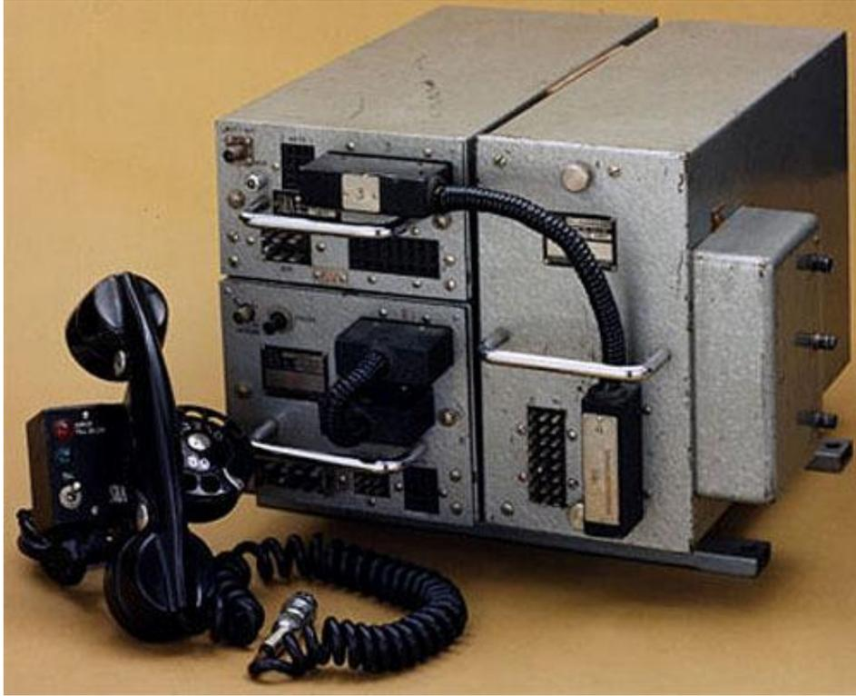
**Figura 1: Mobile Telephone System A (MTA)**
