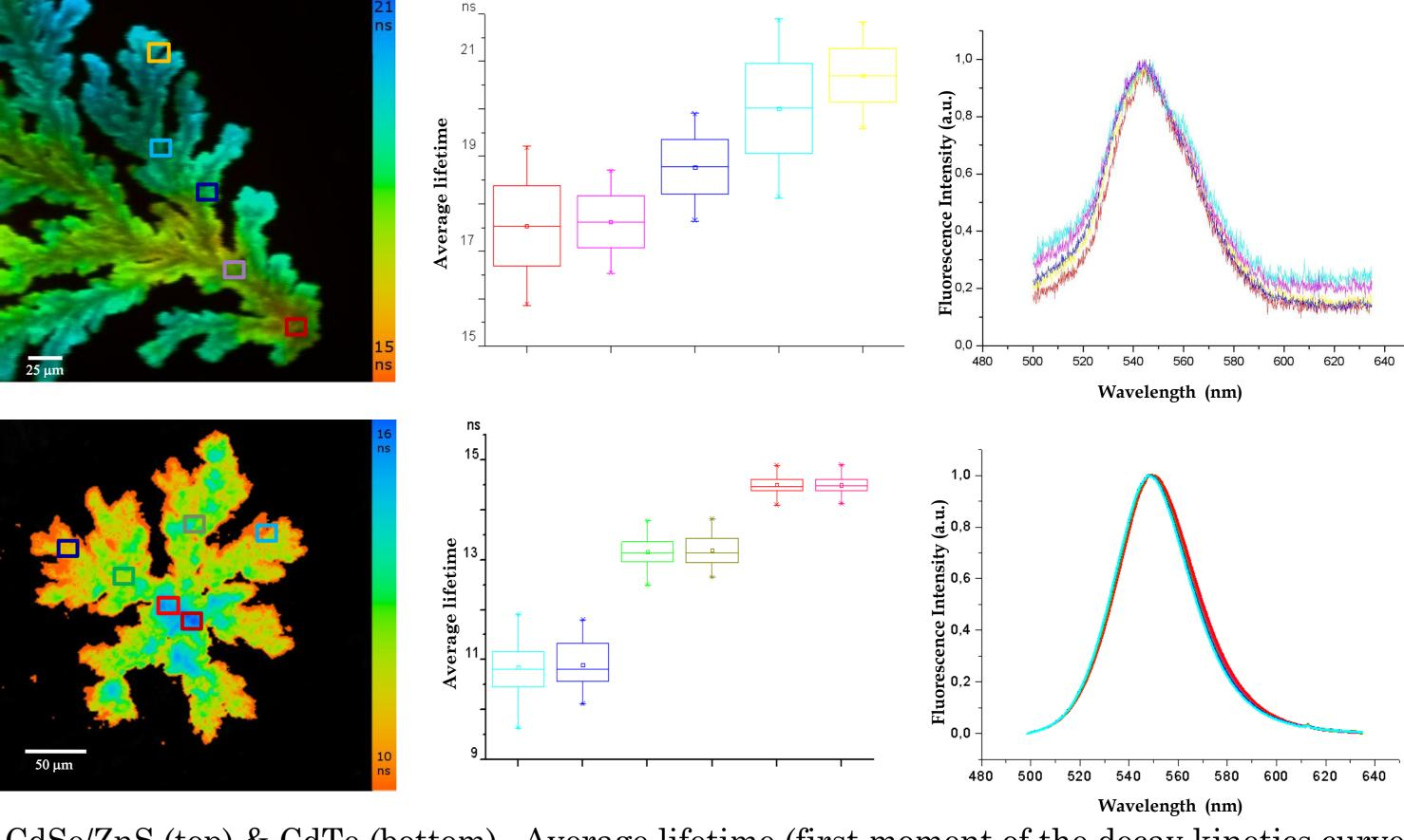
CdSe/ZnS (top) & CdTe (bottom) - Average lifetime (first moment of the decay kinetics curve). The lifetime is color coded (left) according to the scale in nanoseconds (middle). Spatial variation of the average lifetime within selected zones (middle); Fluorescence spectra of the selected zones (right).
