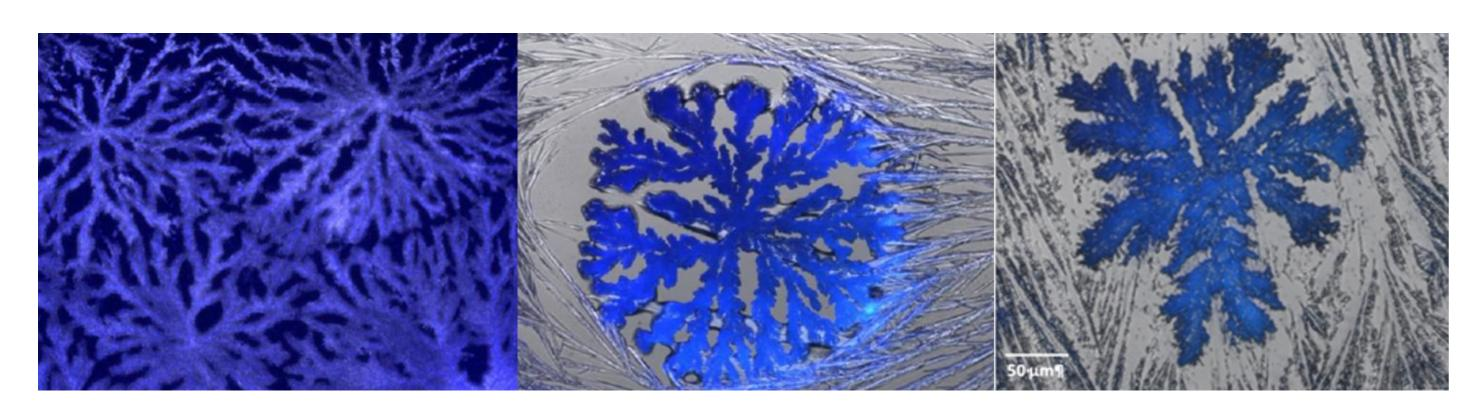
Representative examples of the superstructures built from CdSe/ZnS(left & middle) and CdTe (right) QDs capped with thioglycolic acid, obtained by self-assembling processes [3].
