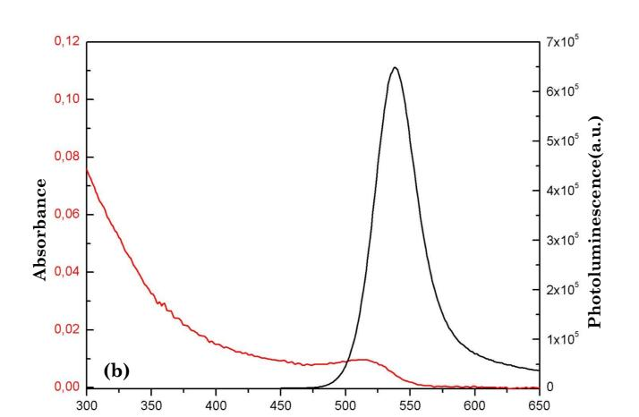
Fluorescence and UV-Vis absorption spectra of colloidal CdSe/ZnS (a) and CdTe (b) QDs capped with thioglycolic acid (TGA), dissolved in water.
