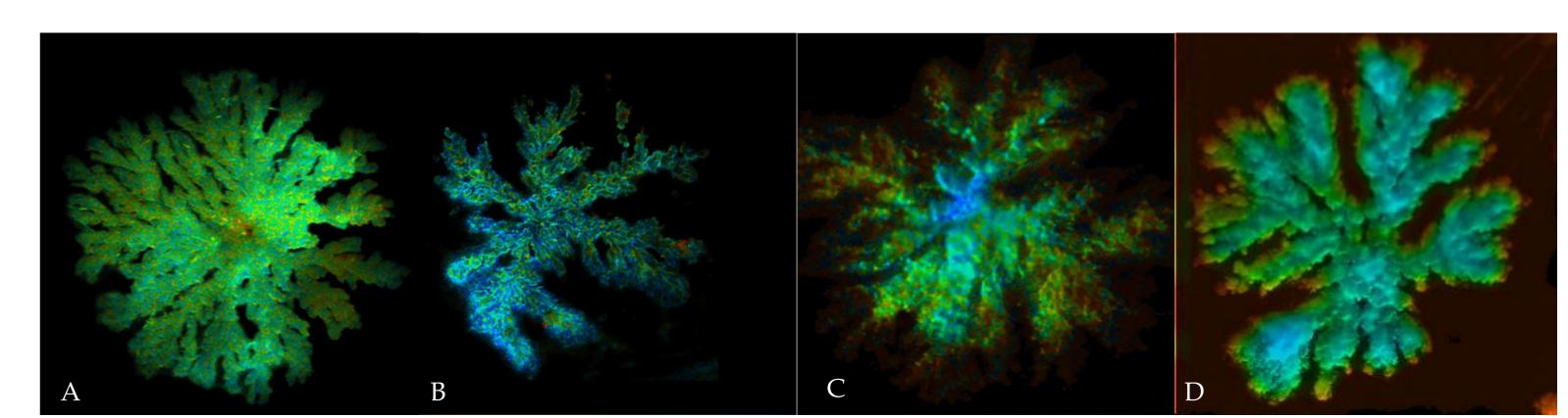
FLIM images from different types of superstructures of CdSe/ZnSe (a,b) & CdTe (c,d) QDs.
