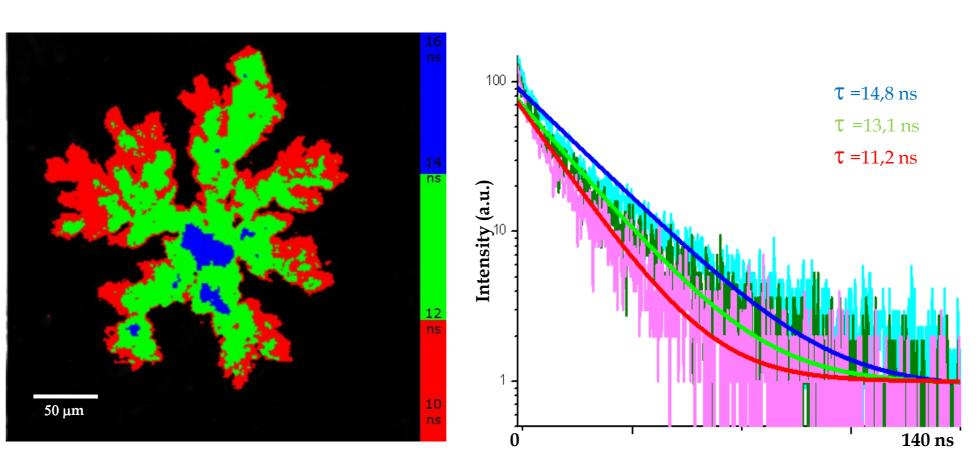
Average lifetime (first moment of the decay kinetics curve). The lifetime is color coded according to ranges of 2 nanoseconds. The excitation wavelength was 400 nm and emission was collected at 545 nm (left); Examples of decay kinetics are given for representative points in each zone (right).
