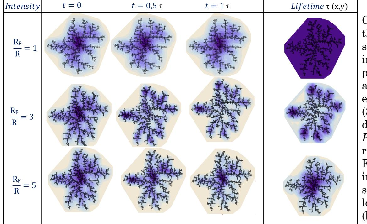
Calculated maps of the emission intendifferent instants after the pulse (2-nd column) and the effective lifetime emission (3-rd column) for different ratios of  $R_F/R$  (R is the QD radius).
