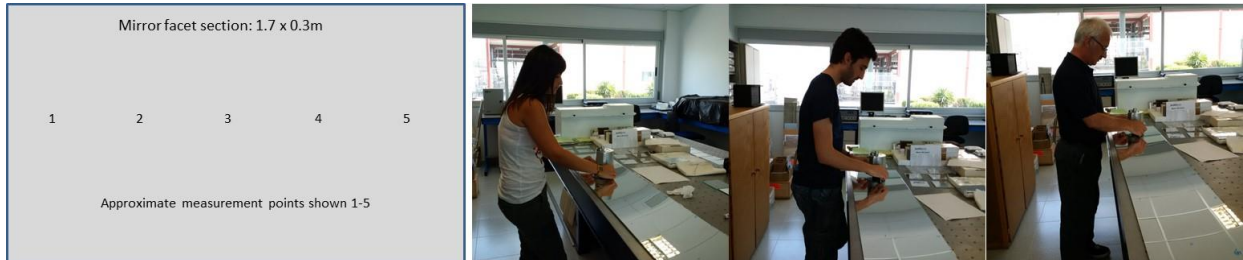
Fig 2. Gage R&R showing measurement positions and three observers using the D&S reflectometer.
