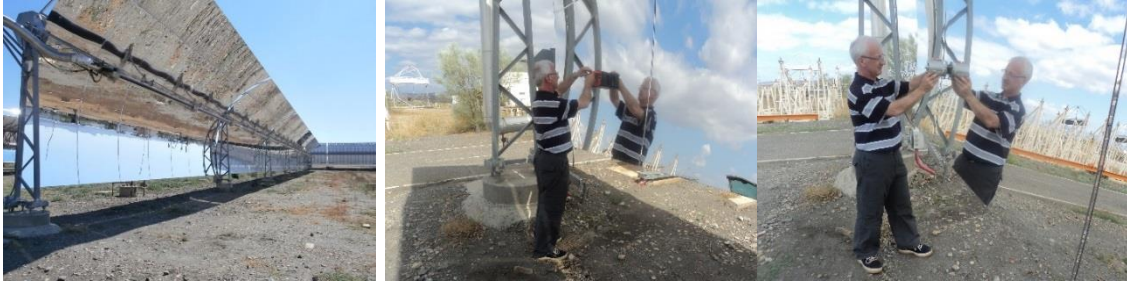
Fig. 3. The PTC line (left) with Condor (center) and D&S (right) reflectance measurements being taken.
