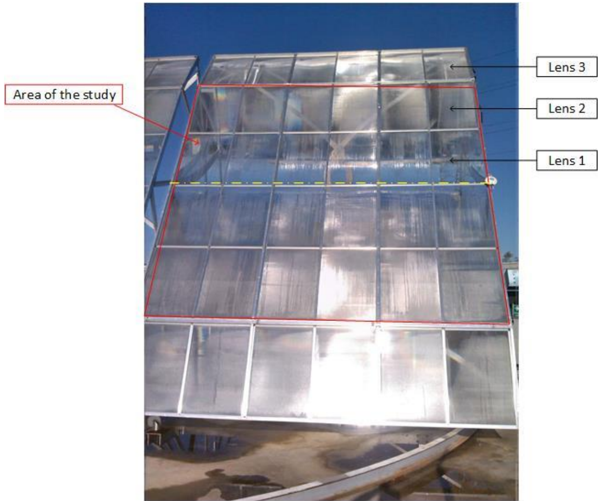
Figure 3: Description of the three section of the optical system. The yellow line represent the axis of symmetry.
