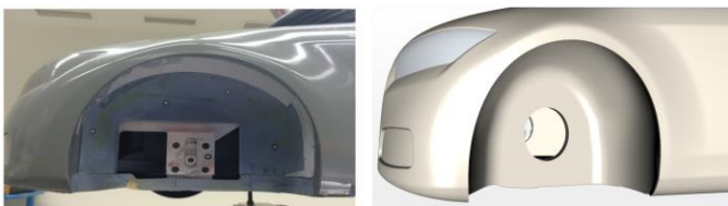
Figure 3. Wheel arch openings showing difference between experimental square baseline [13] and CAD geometry circular opening
